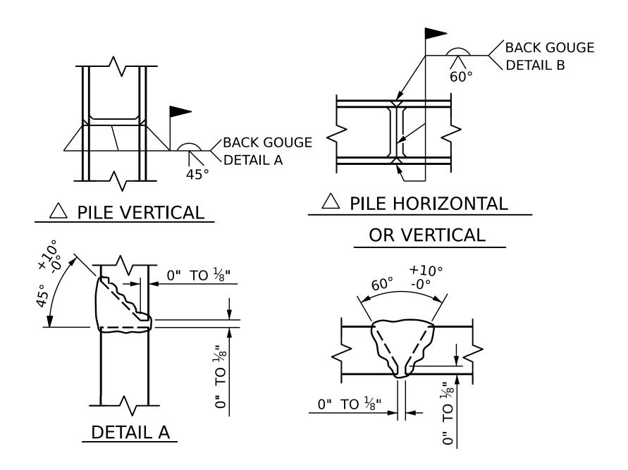
△ POSITION OF PILE DURING WELDING.
