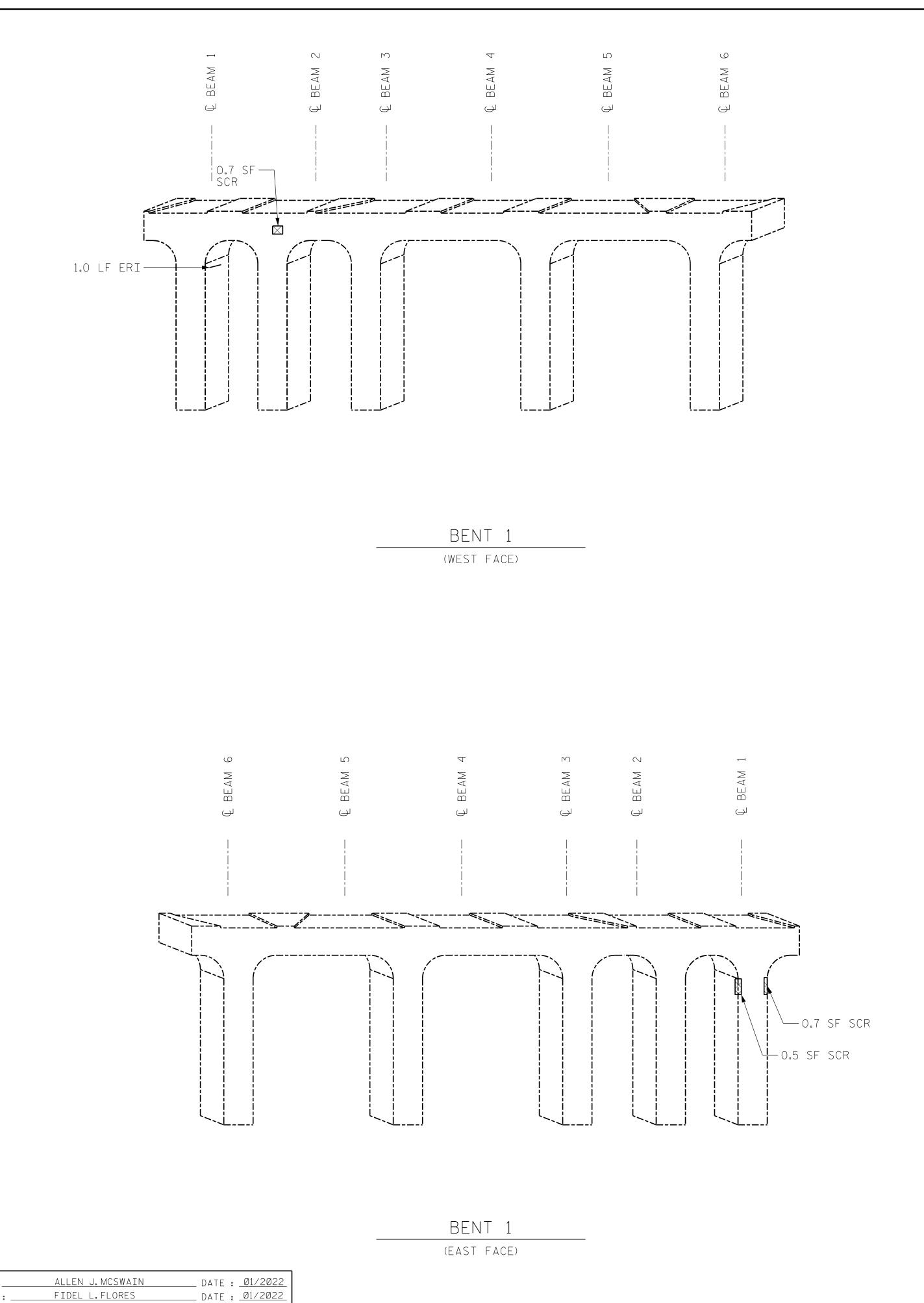
LEGEND AS-BUILT REPAIR QUANTITY TABLE QUANTITIES CONCRETE REPAIR AREA (CR) ACTUAL ESTIMATE SHOTCRETE REPAIR AREA (SCR) SHOTCRETE REPAIRS EPOXY RESIN INJECTION (ERI) CAP/BACKWALL 0.7 0.3 COLUMN/PILE 1.2 VOLUME CU.FT. CONCRETE REPAIRS CAP EPOXY RESIN INJECTION LIN.FT. LIN.FT. CAP/BACKWALL \_ COLUMN/PILE 1.0
