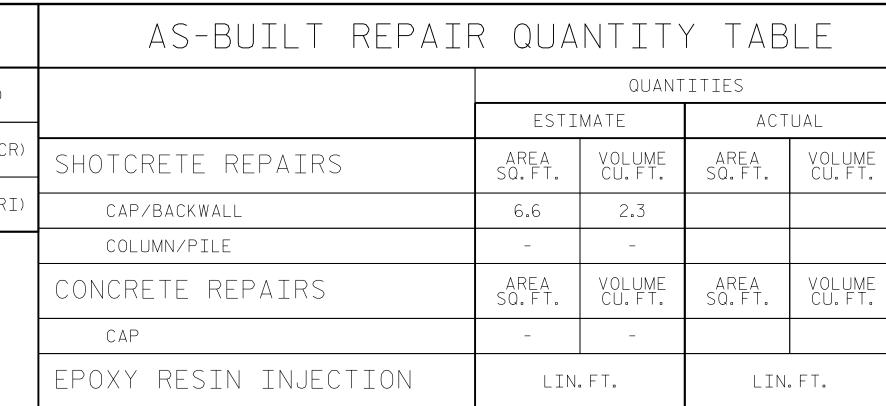
VALUES IN CHART REPRESENT ESTIMATED REPAIR TOTALS AFTER REMOVAL OF UNSOUND CONCRETE. MINIMUM OF 1"BEHIND REBAR AND MINIMUM 2"CLEARANCE TO SAWCUT. FOR REPAIR DETAILS, SEE "CONCRETE RESTORATION DETAILS" SHEETS.
