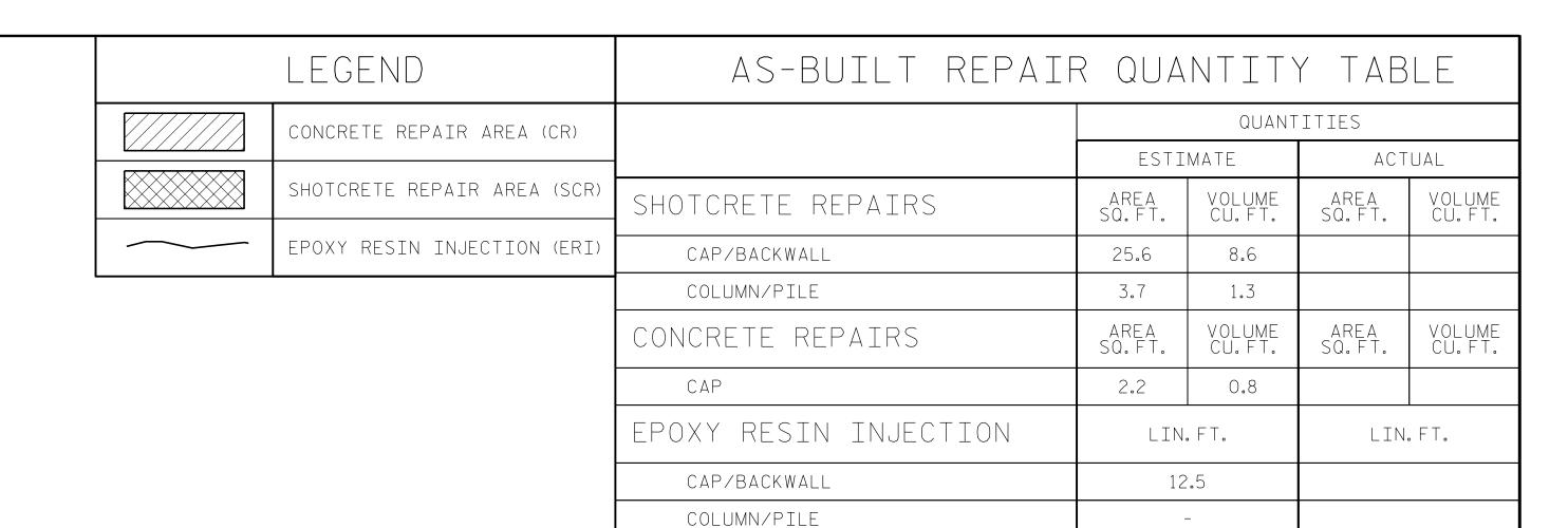
VALUES IN CHART REPRESENT ESTIMATED REPAIR TOTALS AFTER REMOVAL OF UNSOUND CONCRETE. MINIMUM OF 1"BEHIND REBAR AND MINIMUM 2"CLEARANCE TO SAWCUT. FOR REPAIR DETAILS, SEE "CONCRETE RESTORATION DETAILS" SHEETS.
