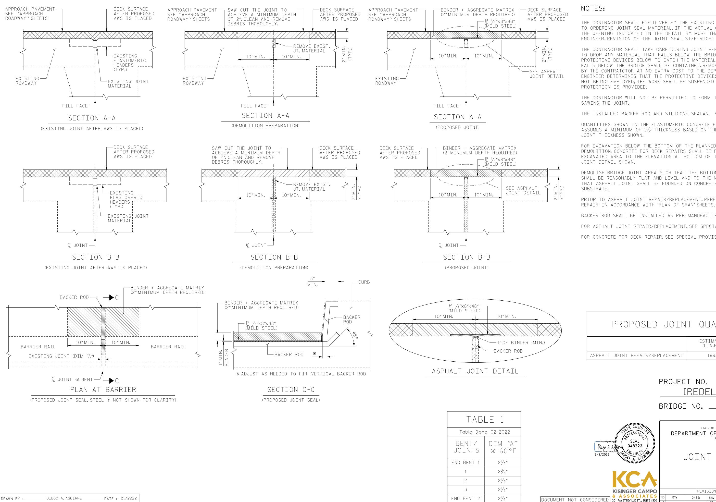
THE CONTRACTOR SHALL FIELD VERIFY THE EXISTING JOINT OPENING PRIOR TO ORDERING JOINT SEAL MATERIAL. IF THE ACTUAL OPENING VARIES FROM THE OPENING INDICATED IN THE DETAIL BY MORE THAN  $\frac{1}{4}$ , NOTIFY THE ENGINEER. REVISION OF THE JOINT SEAL SIZE MIGHT BE NECESSARY.
