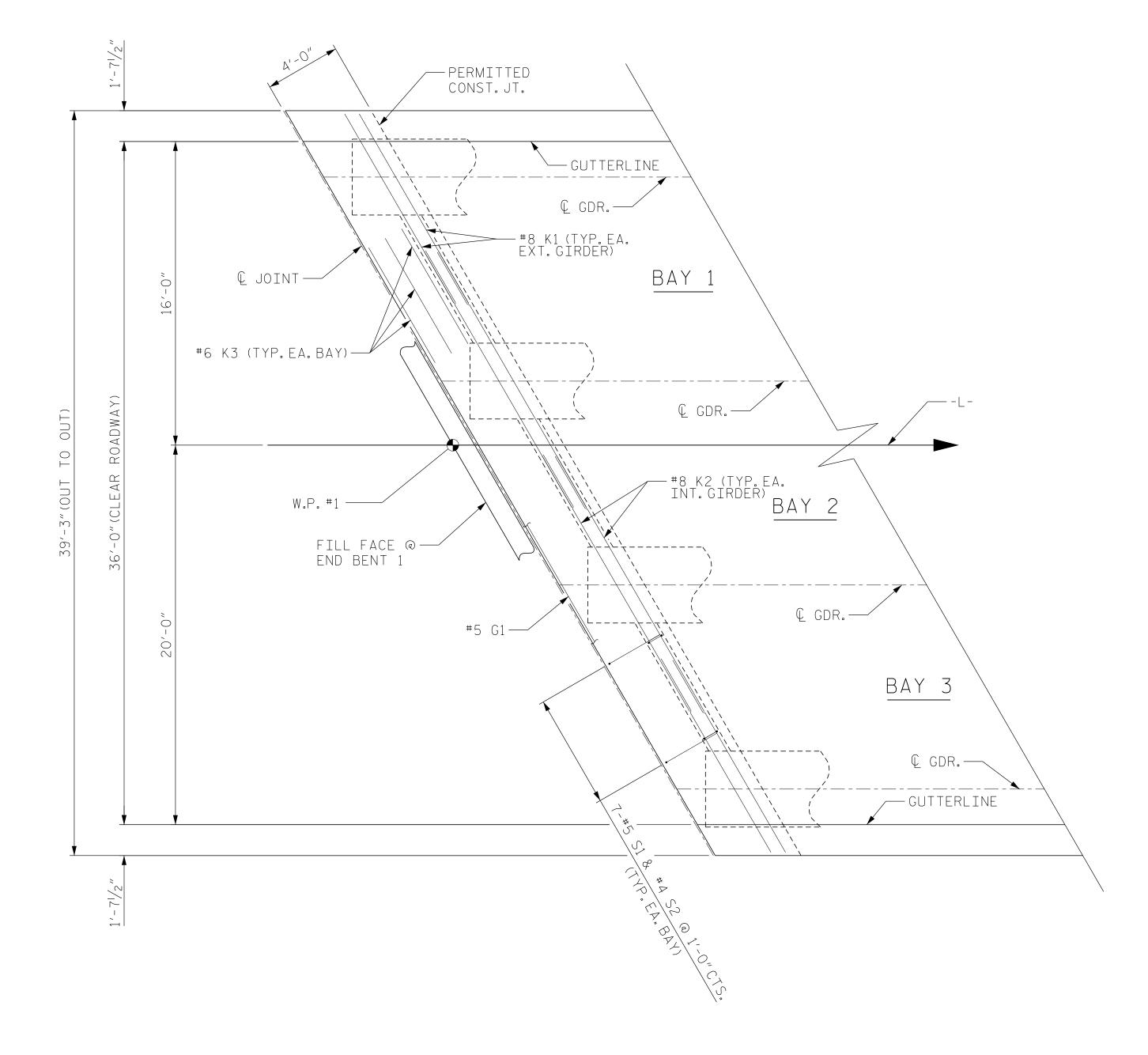
END BENT DIAPHRAGM ENLARGEMENT
