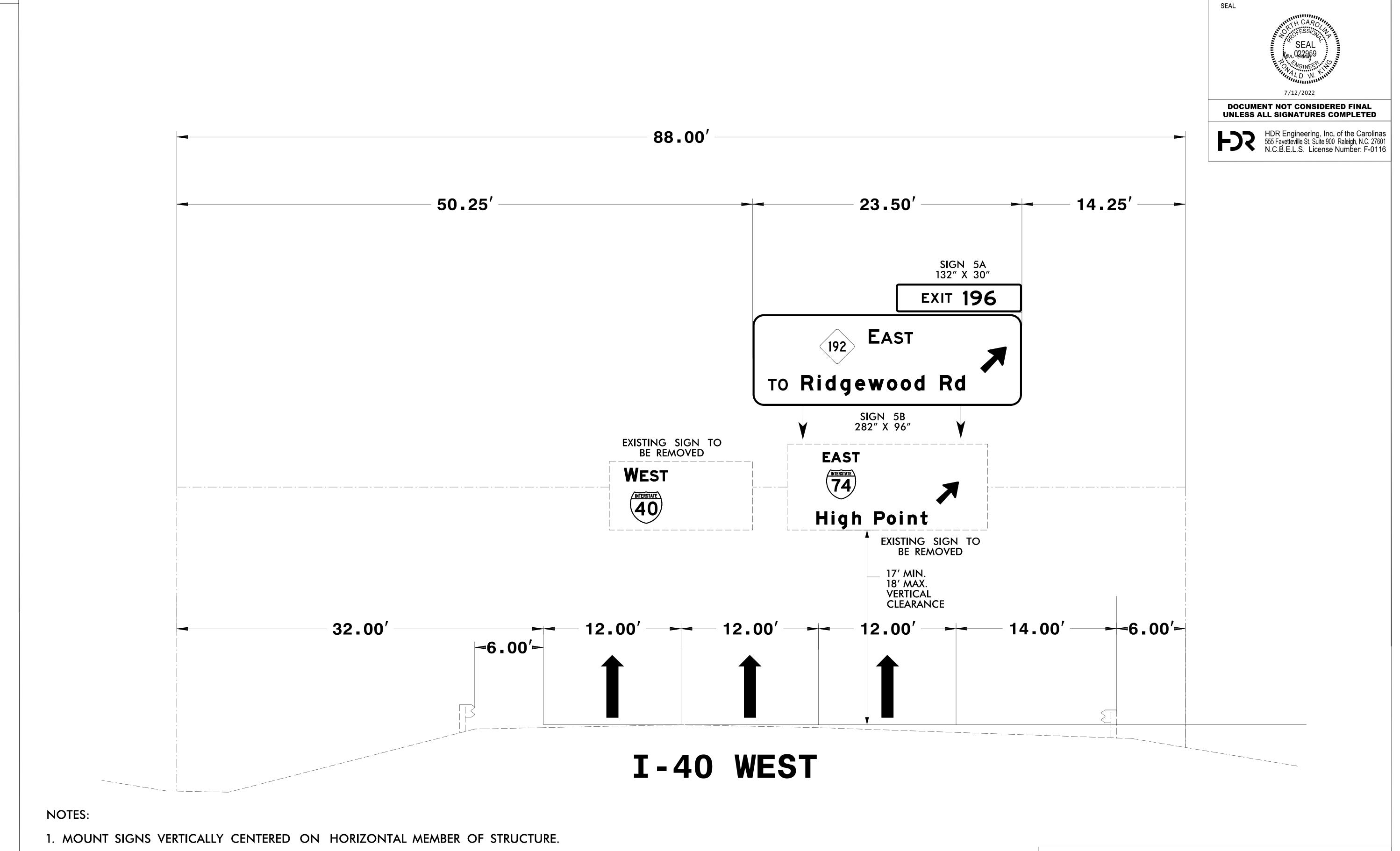
2. SIGN HANGERS AND ATTACHMENT HARDWARE SHALL BE PROVIDED AND INSTALLED ON THE ASSEMBLY TO ACCOMMODATE ALL SIGNS SHOWN IN THIS PLAN SHEET.
