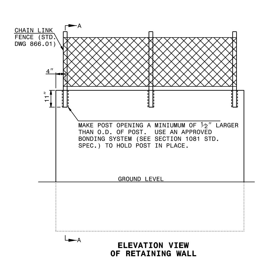
EMBED CHAIN LINK FENCE 11" INTO PROPOSED WALL IN A SLEEVE OR BLOCKOUT WITH EPOXY OR CONCRETE GROUT ANCHORING SYSTEM. PRE-MEASURE AND CENTER THE PROPOSED FENCE ON TOP OF WALL FOR POST SPACINGS. IFF DRILLING THE HOLES FOR POSTS, USE A ROTARY DRILL TO DRILL HOLES IN THE CONCRETE. NO IMPACT DRILLS WILL BE ALLOWED, TO ELIMINATE ANY POSSIBILITY OF STRUCTURAL DAMAGES TO THE PROPOSED WALL.
