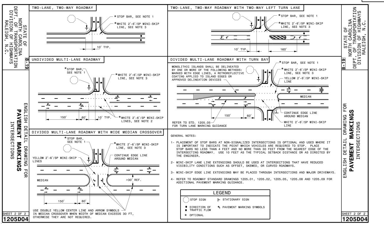
REVISED PAVEMENT MARKING ROADWAY STANDARD DRAWING
