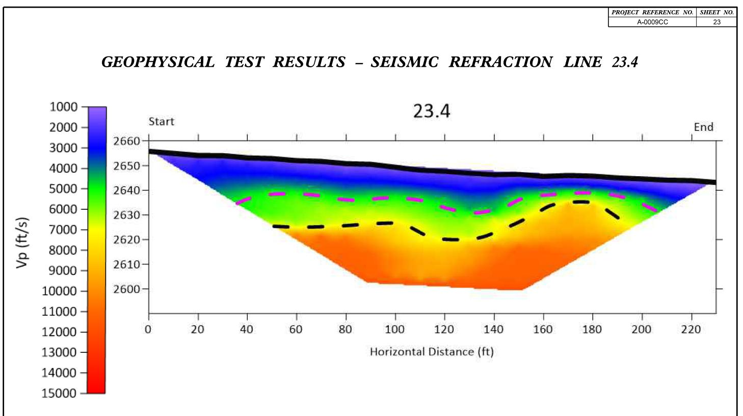
GEOPHYSICAL TESTING PERFORMED BY GEL SOLUTIONS. REFERENCE "SEISMIC REFRACTION SURVEY FOR EVALUATION OF ROCK" DATED 10/01/2021 CG2 ESTIMATED WAVE SPEED FOR WEATHERED ROCK: 4,500 FT/SEC CG2 ESTIMATED WAVE SPEED FOR CRYSTALLINE ROCK: 7,500 FT/SEC
