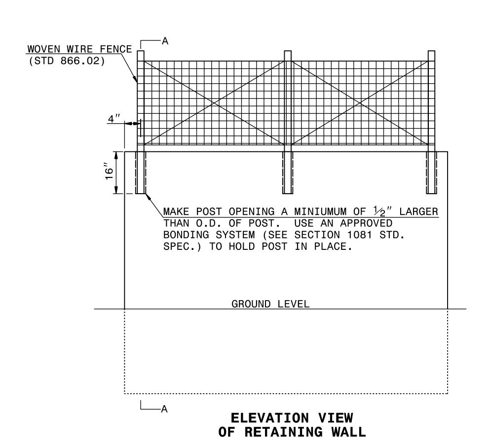
EMBED WOVEN WIRE FENCE 16" INTO PROPOSED WALL IN A SLEEVE OR BLOCKOUT WITH EPOXY OR CONCRETE GROUT ANCHORING SYSTEM. PRE-MEASURE AND CENTER THE PROPOSED FENCE ON TOP OF WALL FOR POST SPACINGS. IF DRILLING THE HOLES FOR POSTS, USE A ROTARY DRILL TO DRILL HOLES IN THE CONCRETE. NO IMPACT DRILLS WILL BE ALLOWED, TO ELIMINATE ANY POSSIBILITY OF STRUCTURAL DAMAGES TO THE PROPOSED WALL.
