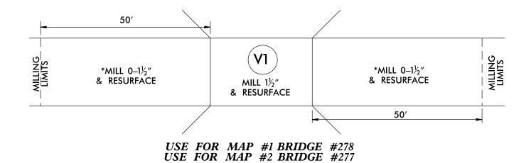
\* MILLING FOR APPROACHES SHALL BE PAID FOR UNDER INCIDENTAL MILLING
