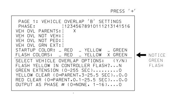
PAGE 1: VEHICLE OVERLAP 'D' SETTINGS 12345678910111213141516 VEH OVL PARENTS: | VEH OVL NOT VEH: VEH OVL NOT PED: | VEH OVL GRN EXT: | STARTUP COLOR: \_ RED \_ YELLOW \_ GREEN FLASH COLORS: \_ RED \_ YELLOW X GREEN NOTICE SELECT VEHICLE OVERLAP OPTIONS: (Y/N) GREEN FLASH YELLOW IN CONTROLLER FLASH?...N FLASH GREEN EXTENSION (0-255 SEC)..... YELLOW CLEAR (0=PARENT,3-25.5 SEC)..0.0 RED CLEAR (0=PARENT, 0.1-25.5 SEC)...0.0 OUTPUT AS PHASE # (0=NONE, 1-16)....0
