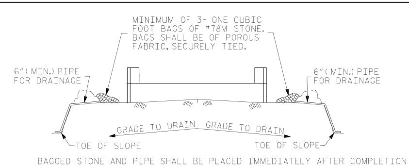
OF END BENT EXCAVATION. PIPE MAY BE EITHER CONCRETE, CORRUGATED STEEL, CORRUGATED ALUMINUM ALLOY, OR CORRUGATED PLASTIC. PERFORATED PIPE WILL NOT BE ALLOWED.
