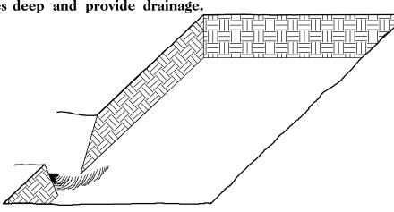
3. Backfill the trench with 2 inches well rotted sawdust. Place a 2 inch layer of well rotted sawdust at a sloping angle
