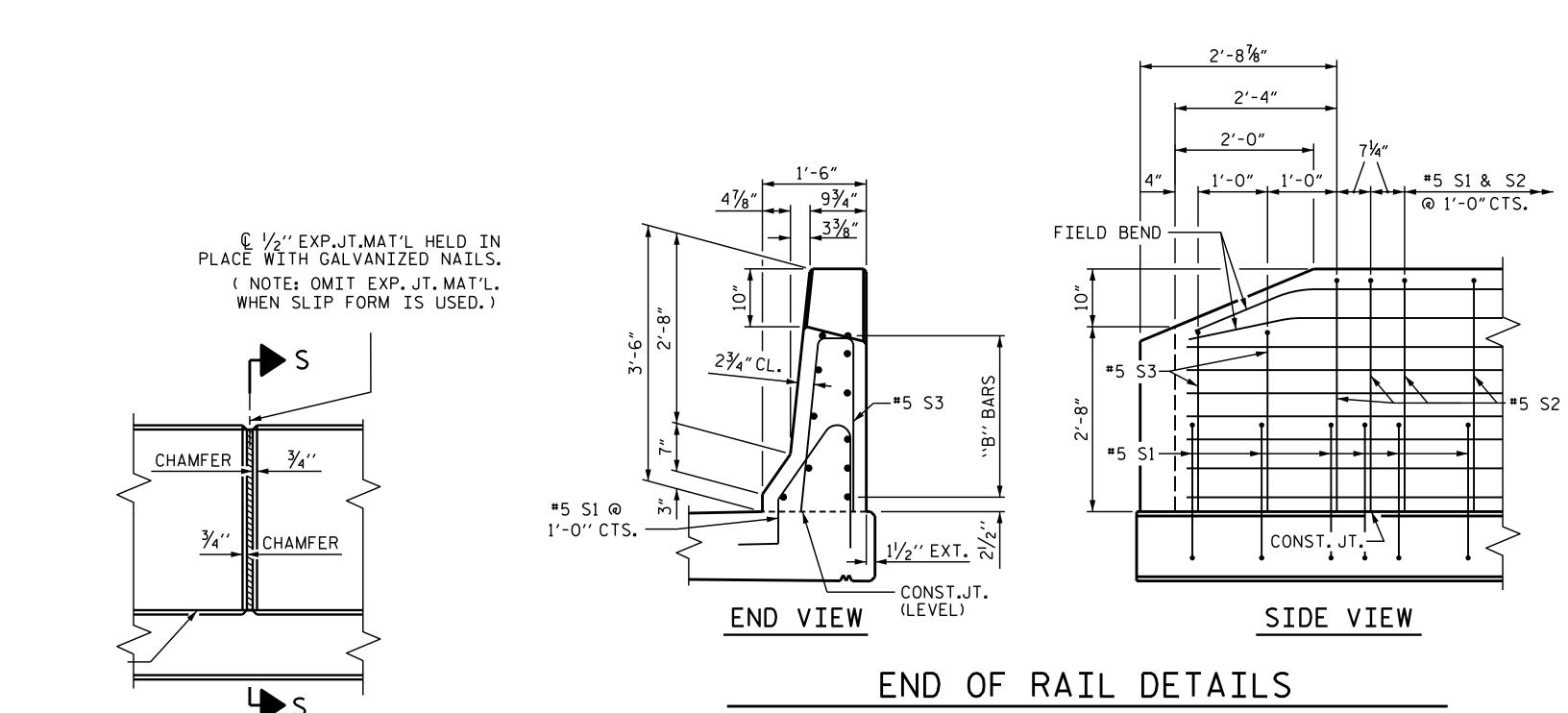
THE BARRIER RAIL IN EACH SPAN SHALL NOT BE CAST UNTIL ALL SLAB CONCRETE IN THAT SPAN HAS BEEN CAST AND HAS REACHED A MINIMUM COMPRESSIVE STRENGTH OF 3,000 PSI.
