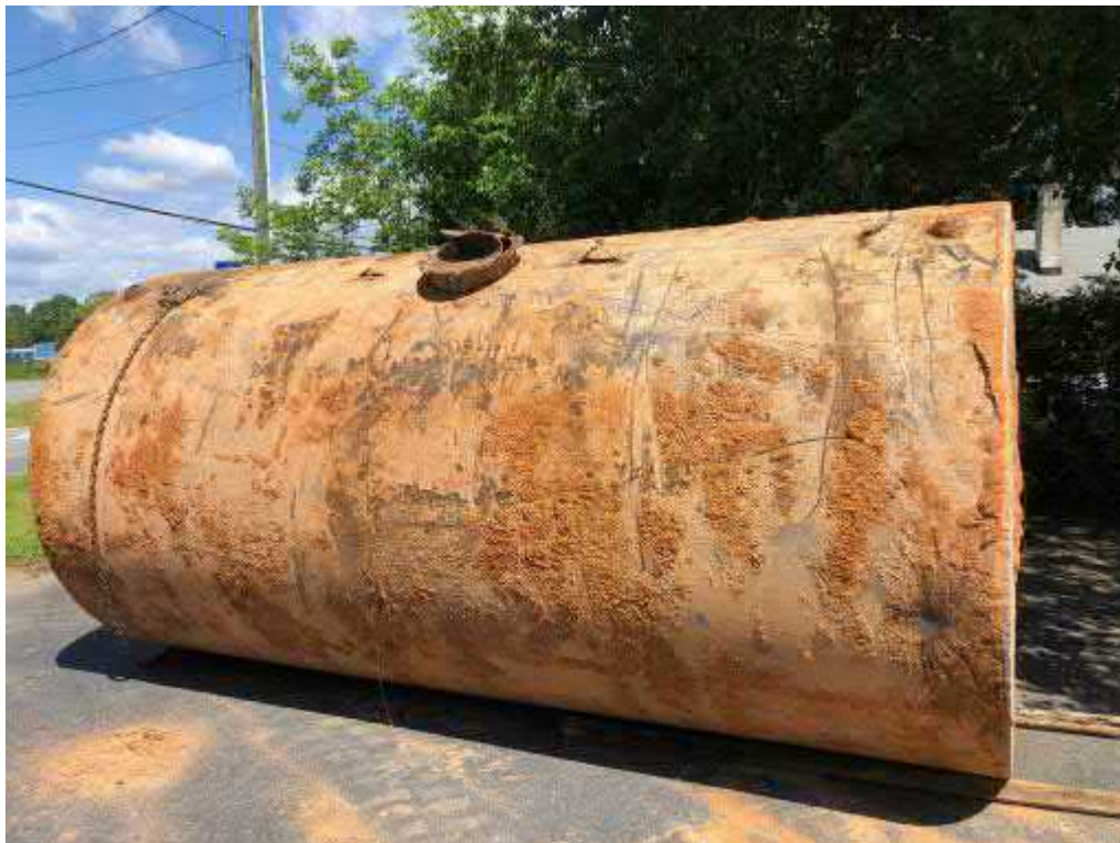
Photo 6 - View of 6,000-gallon UST after excavation
