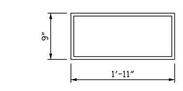
E4 (40 REQ'D) PLAN VIEW OF ELASTOMERIC BEARING TYPE V
