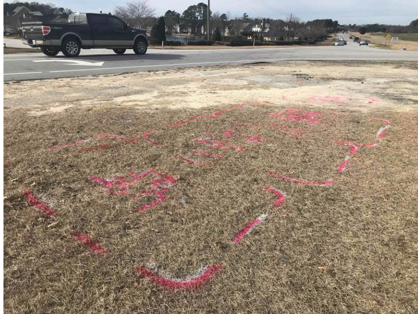
Photo #3 View of the four probable USTs identified in the geophysical investigation; facing northwest.
