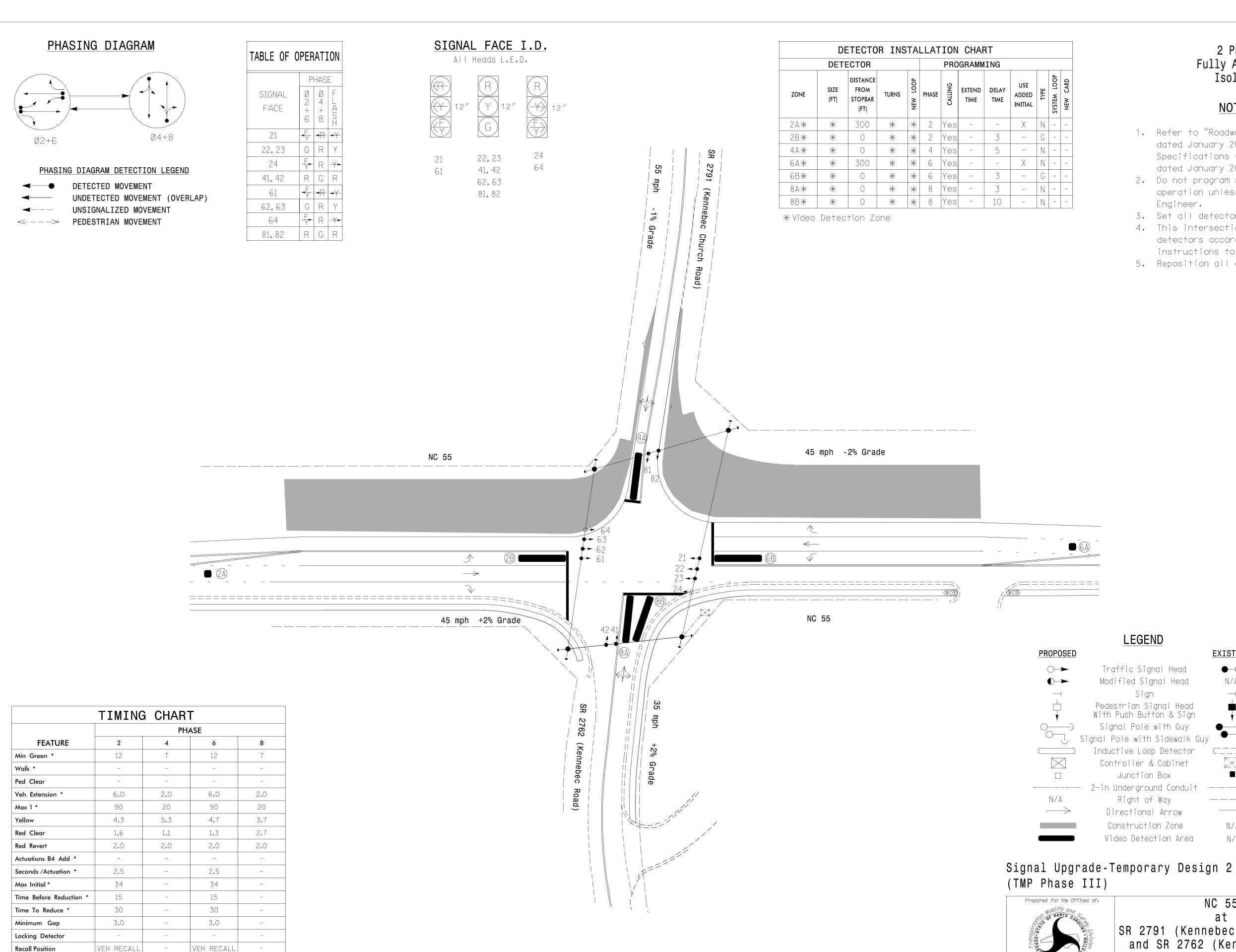
\* These values may be field adjusted. Do not adjust Min Green and Extension times for phases 2 and 6 lower than what is shown. Min Green for all other phases should not be lower than 4 seconds.
