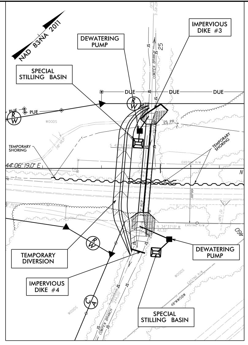
CONSTRUCTION SEQUENCE STA. 24 + 79 -Y3-FOR PROPOSED (2) 8' X 7' RCBC
