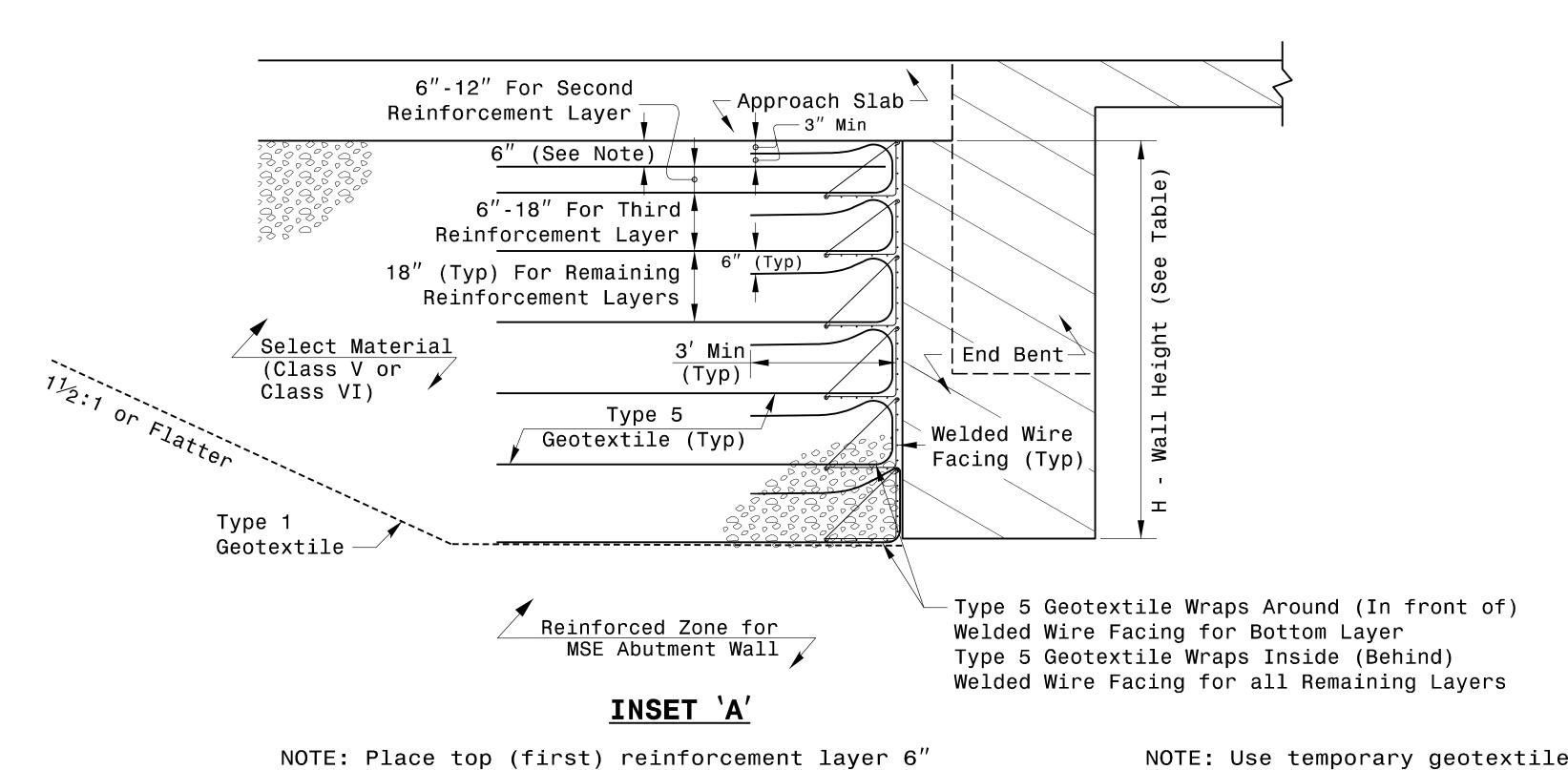
NOTE: Use temporary geotextile wall to construct approach embankments to finished grade before observing waiting periods, driving bridge foundation piles, or constructing end bent caps.
