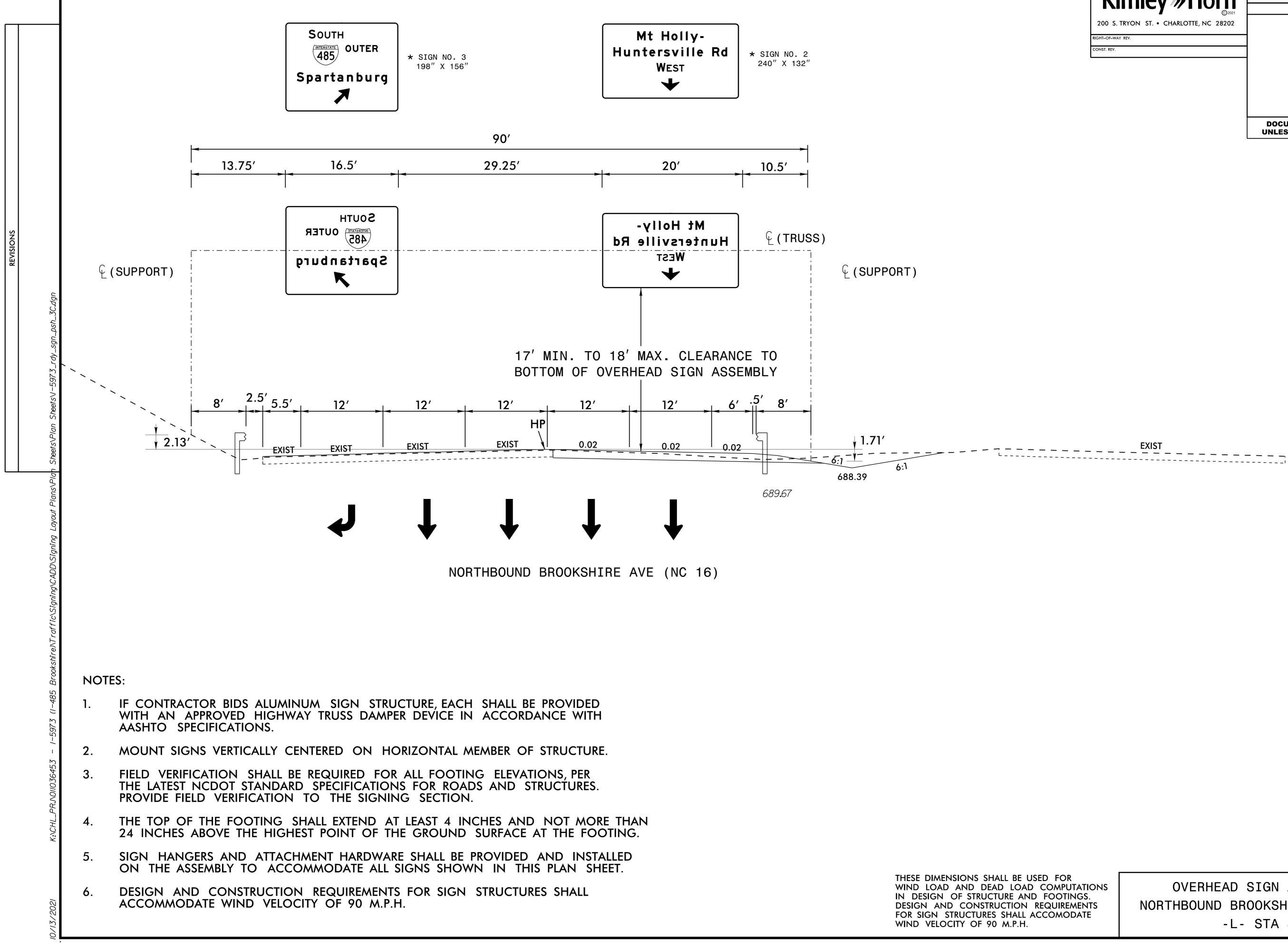
THESE DIMENSIONS SHALL BE USED FOR WIND LOAD AND DEAD LOAD COMPUTATIONS IN DESIGN OF STRUCTURE AND FOOTINGS. DESIGN AND CONSTRUCTION REQUIREMENTS FOR SIGN STRUCTURES SHALL ACCOMODATE
