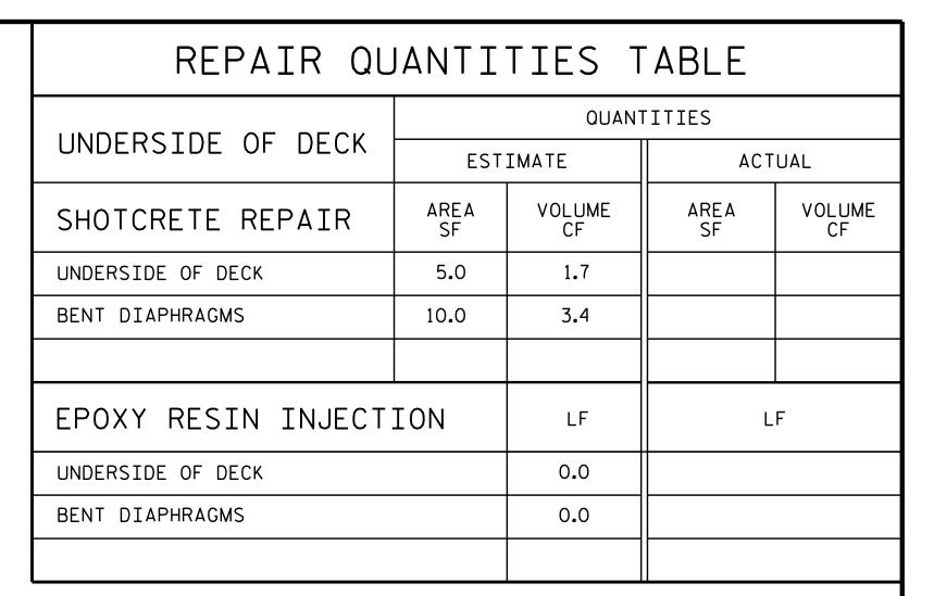
VALUES IN CHART REPRESENT ESTIMATED REPAIR QUANTITIES AFTER REMOVAL OF UNSOUND CONCRETE, MIN. OF 1"BEHIND REBAR AND MIN. 1"CL TO SAWCUT. SEE REPAIR DETAILS.
