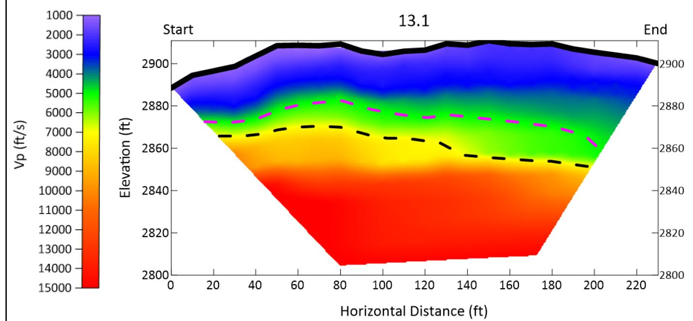
GEOPHYSICAL TESTING PERFORMED BY GEL SOLUTIONS. REFERENCE "SEISMIC REFRACTION SURVEY FOR EVALUATION OF ROCK" DATED 10/01/2021 CG2 ESTIMATED WAVE SPEED FOR WEATHERED ROCK: 4,500 FT/SEC
