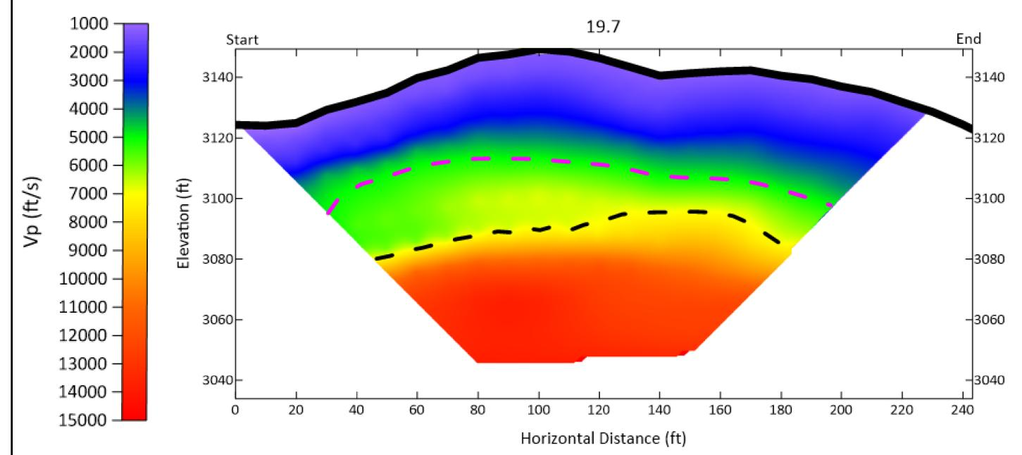
GEOPHYSICAL TESTING PERFORMED BY GEL SOLUTIONS. REFERENCE "SEISMIC REFRACTION SURVEY FOR EVALUATION OF ROCK" DATED 10/01/2021 CG2 ESTIMATED WAVE SPEED FOR WEATHERED ROCK: 4,500 FT/SEC
