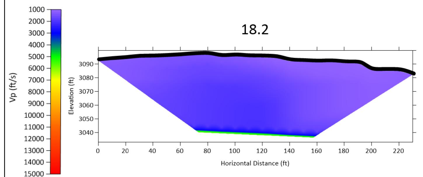
GEOPHYSICAL TESTING PERFORMED BY GEL SOLUTIONS. REFERENCE "SEISMIC REFRACTION SURVEY FOR EVALUATION OF ROCK" DATED 10/01/2021 CG2 ESTIMATED WAVE SPEED FOR WEATHERED ROCK: 4,500 FT/SEC
