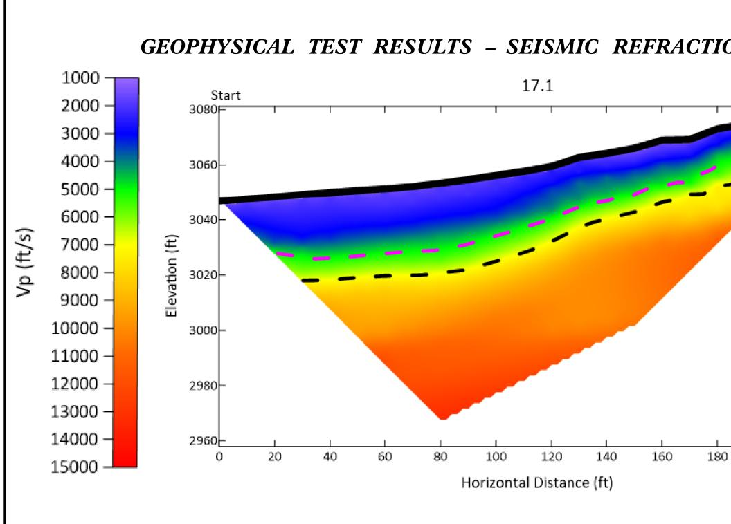
GEOPHYSICAL TESTING PERFORMED BY GEL SOLUTIONS. REFERENCE "SEISMIC REFRACTION SURVEY FOR EVALUATION OF ROCK" DATED 10/01/2021 CG2 ESTIMATED WAVE SPEED FOR WEATHERED ROCK: 4,500 FT/SEC CG2 ESTIMATED WAVE SPEED FOR CRYSTALLINE ROCK: 7,500 FT/SEC
