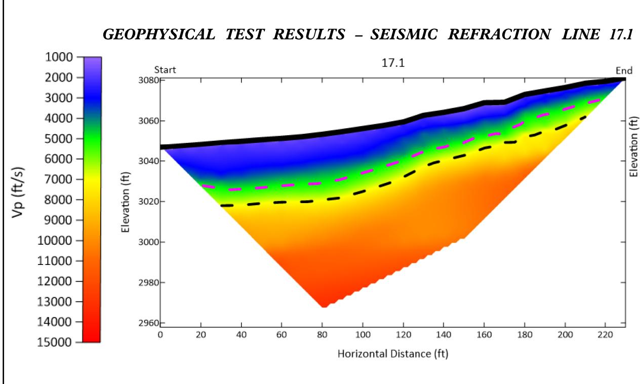
GEOPHYSICAL TESTING PERFORMED BY GEL SOLUTIONS. REFERENCE "SEISMIC REFRACTION SURVEY FOR EVALUATION OF ROCK" DATED 10/01/2021 CG2 ESTIMATED WAVE SPEED FOR WEATHERED ROCK: 4,500 FT/SEC CG2 ESTIMATED WAVE SPEED FOR CRYSTALLINE ROCK: 7,500 FT/SEC
