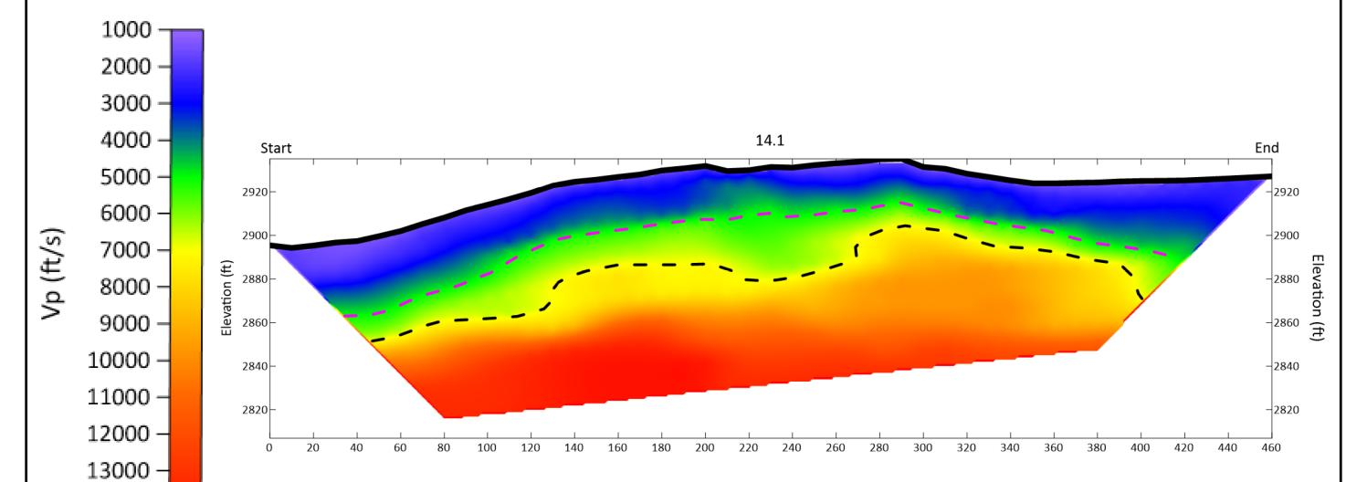
GEOPHYSICAL TESTING PERFORMED BY GEL SOLUTIONS. REFERENCE "SEISMIC REFRACTION SURVEY FOR EVALUATION OF ROCK" DATED 10/01/2021 CG2 ESTIMATED WAVE SPEED FOR WEATHERED ROCK: 4,500 FT/SEC
