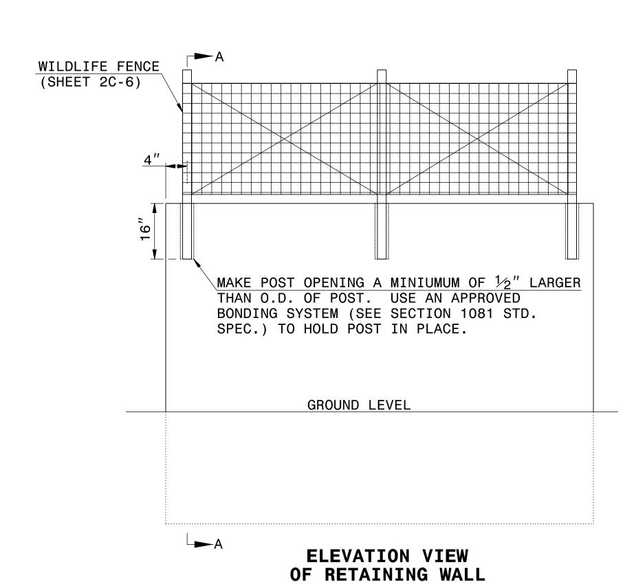
EMBED WILDLIFE FENCE 16" INTO PROPOSED WALL IN A SLEEVE OR BLOCKOUT WITH EPOXY OR CONCRETE GROUT ANCHORING SYSTEM.
