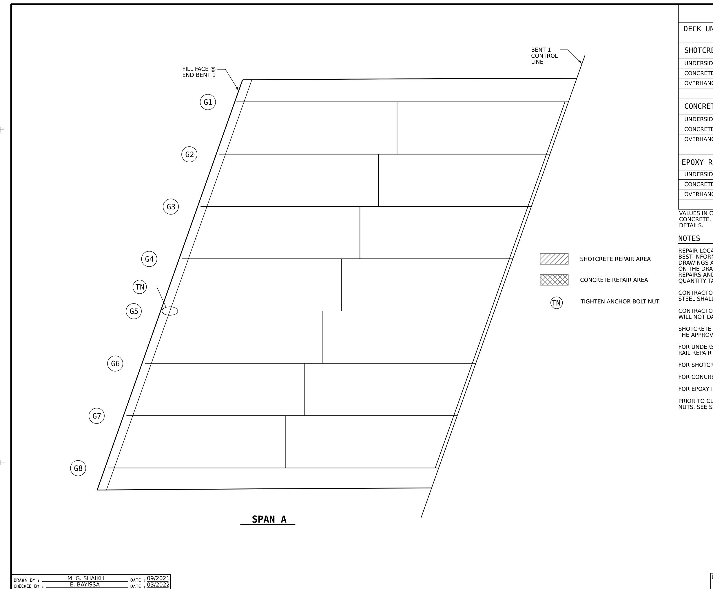
AS-BUILT REPAIR QUANTITY TABLE QUANTITIES DECK UNDERSIDE REPAIRS SPAN A ACTUAL **ESTIMATE** AREA VOLUME VOLUME AREA SHOTCRETE REPAIRS SF 0.0 UNDERSIDE OF DECK 0.0 CONCRETE DIAPHRAGM 0.0 0.0 OVERHANG 0.0 0.0 AREA VOLUME AREA VOLUME CONCRETE REPAIRS SF 0.0 UNDERSIDE OF DECK 0.0 CONCRETE DIAPHRAGM 0.0 0.0 0.0 OVERHANG 0.0 EPOXY RESIN INJECTION LIN. FT. LIN. FT. UNDERSIDE OF DECK 0.0 CONCRETE DIAPHRAGM 0.0 0.0 OVERHANG
