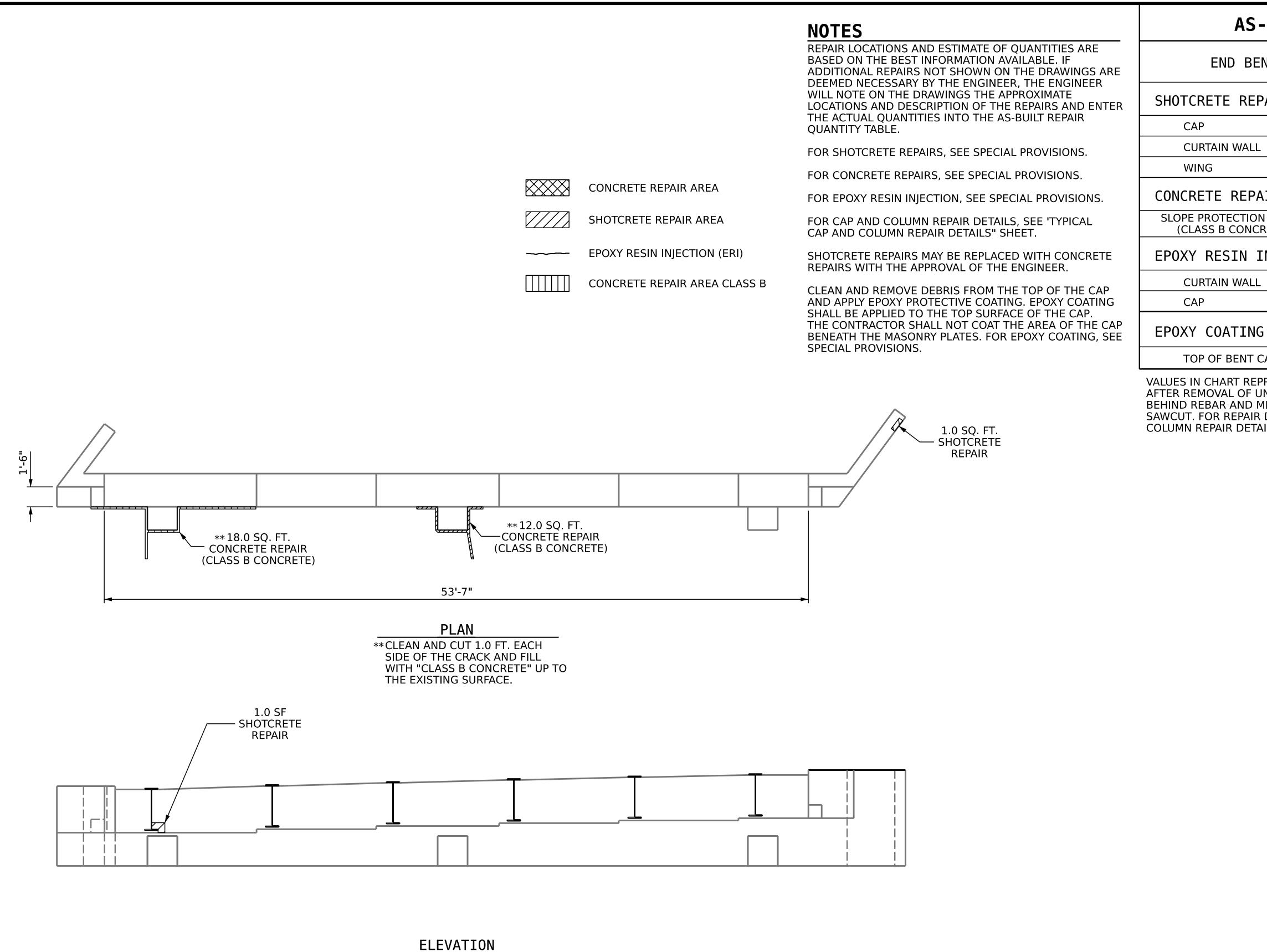
AS-BUILT REPAIR QUANTITY TABLE QUANTITIES END BENT 2 **ESTIMATE** ACTUAL AREA VOLUME AREA VOLUME SHOTCRETE REPAIRS SQ FT. SQ. FT. CU. FT. CU. FT. CAP 0.0 0.0 0.5 CURTAIN WALL 1.0 WING 0.5 1.0 **VOLUME** AREA VOLUME AREA **CONCRETE REPAIRS** SQ. FT. CU. FT. SQ. FT. CU. FT. SLOPE PROTECTION REPAIR 30.0 10.0 (CLASS B CONCRETE) EPOXY RESIN INJECTION LIN. FT. LIN. FT. **CURTAIN WALL** 0.0 0.0 CAP
