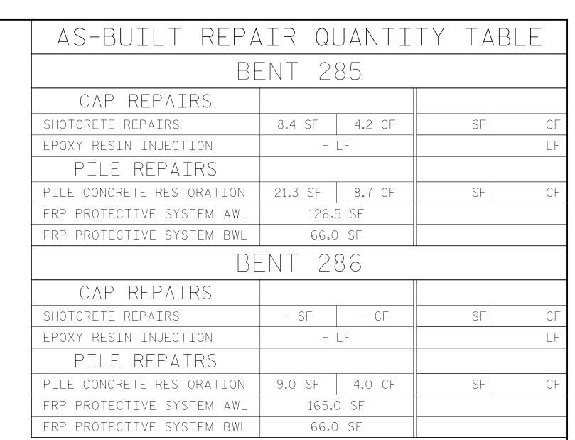
FOR CAP REPAIRS: VALUES IN CHART REPRESENT ESTIMATED REPAIR TOTALS AFTER REMOVAL OF UNSOUND CONCRETE, MIN. OF 1"BEHIND REBAR AND MIN. 2 CL. TO SAWCUT. SEE REPAIR DETAILS.
