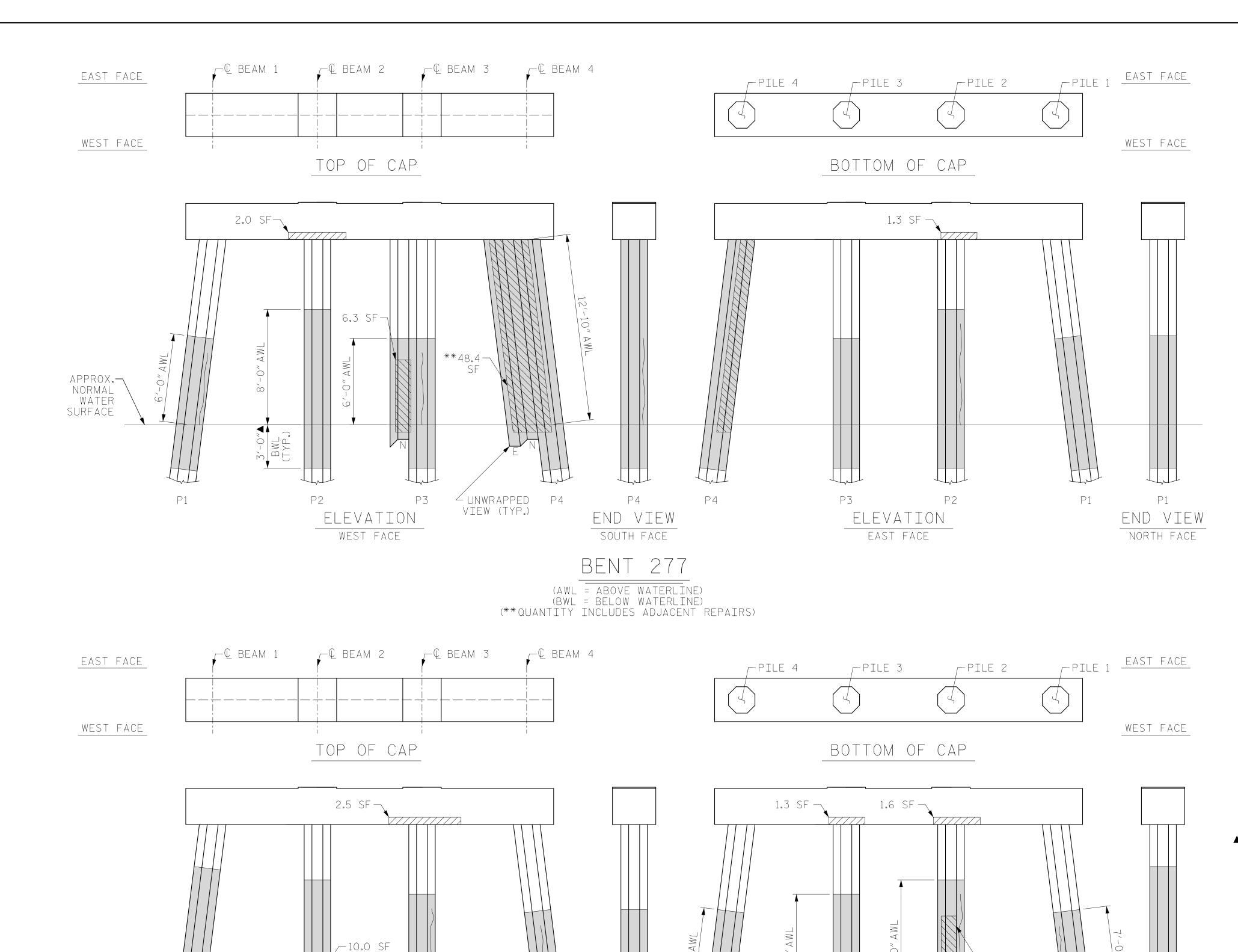
AS-BUILT REPAIR QUANTITY TABLE BENT 277 CAP REPAIRS SF SHOTCRETE REPAIRS 3.3 SF | 1.7 CF EPOXY RESIN INJECTION - LF PILE REPAIRS SF PILE CONCRETE RESTORATION | 54.7 SF | 20.5 CF FRP PROTECTIVE SYSTEM AWL 180.6 SF FRP PROTECTIVE SYSTEM BWL 66.0 SF BENT 278 CAP REPAIRS SF SHOTCRETE REPAIRS 5.4 SF | 2.7 CF - LF EPOXY RESIN INJECTION PILE REPAIRS
