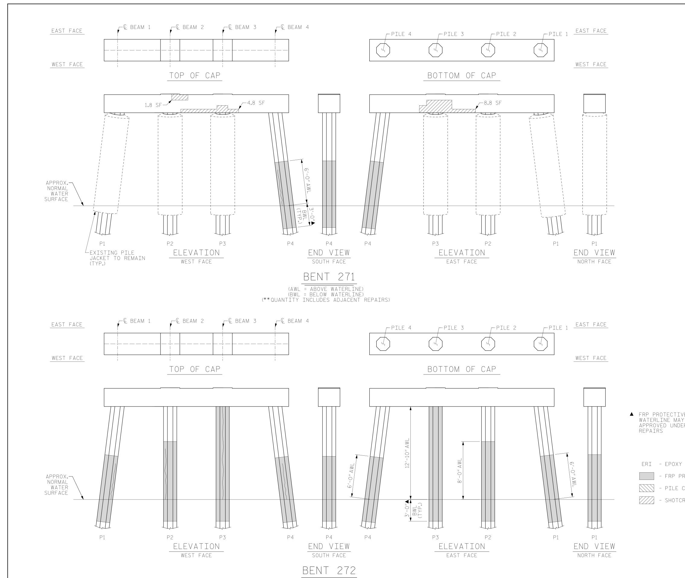
AS-BUILT REPAIR QUANTITY TABLE BENT 271 CAP REPAIRS SF SHOTCRETE REPAIRS 15.4 SF | 7.7 CF EPOXY RESIN INJECTION - LF PILE REPAIRS SF PILE CONCRETE RESTORATION - SF
