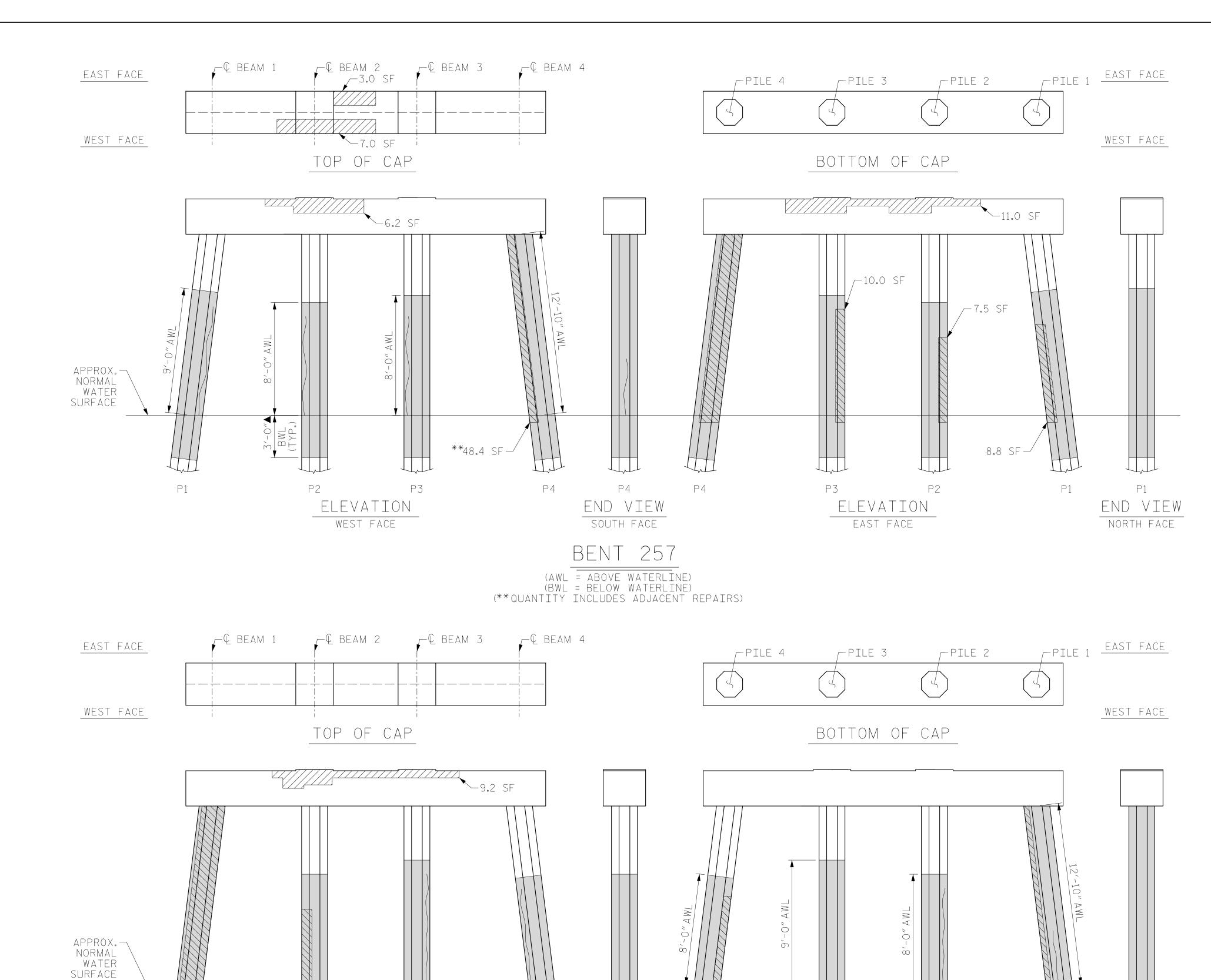
AS-BUILT REPAIR QUANTITY TABLE BENT 257 CAP REPAIRS 27.2 SF | 13.6 CF SF SHOTCRETE REPAIRS EPOXY RESIN INJECTION - LF PILE REPAIRS SF PILE CONCRETE RESTORATION 74.7 SF | 29.0 CF FRP PROTECTIVE SYSTEM AWL 208.1 SF FRP PROTECTIVE SYSTEM BWL 66.0 SF BENT 258 CAP REPAIRS SF SHOTCRETE REPAIRS 9.2 SF 4.6 CF EPOXY RESIN INJECTION - LF PILE REPAIRS PILE CONCRETE RESTORATION 64.7 SF | 24.7 CF SF FRP PROTECTIVE SYSTEM AWL 208.1 SF FRP PROTECTIVE SYSTEM BWL 66.0 SF
