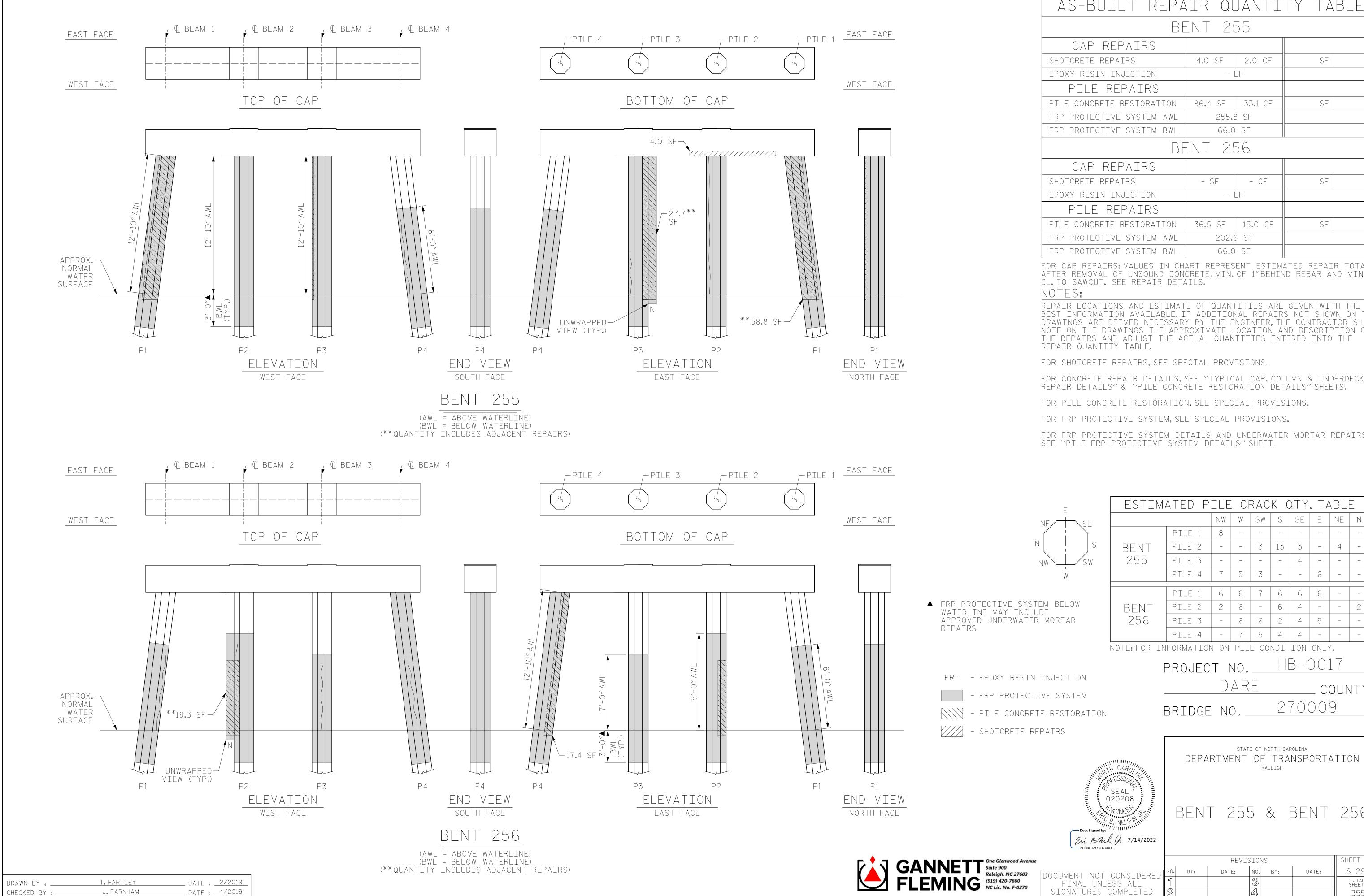
AS-BUILT REPAIR QUANTITY TABLE BENT 255 CAP REPAIRS SF 4.0 SF | 2.0 CF EPOXY RESIN INJECTION - LF PILE REPAIRS PILE CONCRETE RESTORATION | 86.4 SF | 33.1 CF SF FRP PROTECTIVE SYSTEM AWL 255.8 SF FRP PROTECTIVE SYSTEM BWL 66.0 SF BENT 256 CAP REPAIRS SF - SF - CF EPOXY RESIN INJECTION - LF PILE REPAIRS PILE CONCRETE RESTORATION 36.5 SF | 15.0 CF SF FRP PROTECTIVE SYSTEM AWL 202.6 SF
