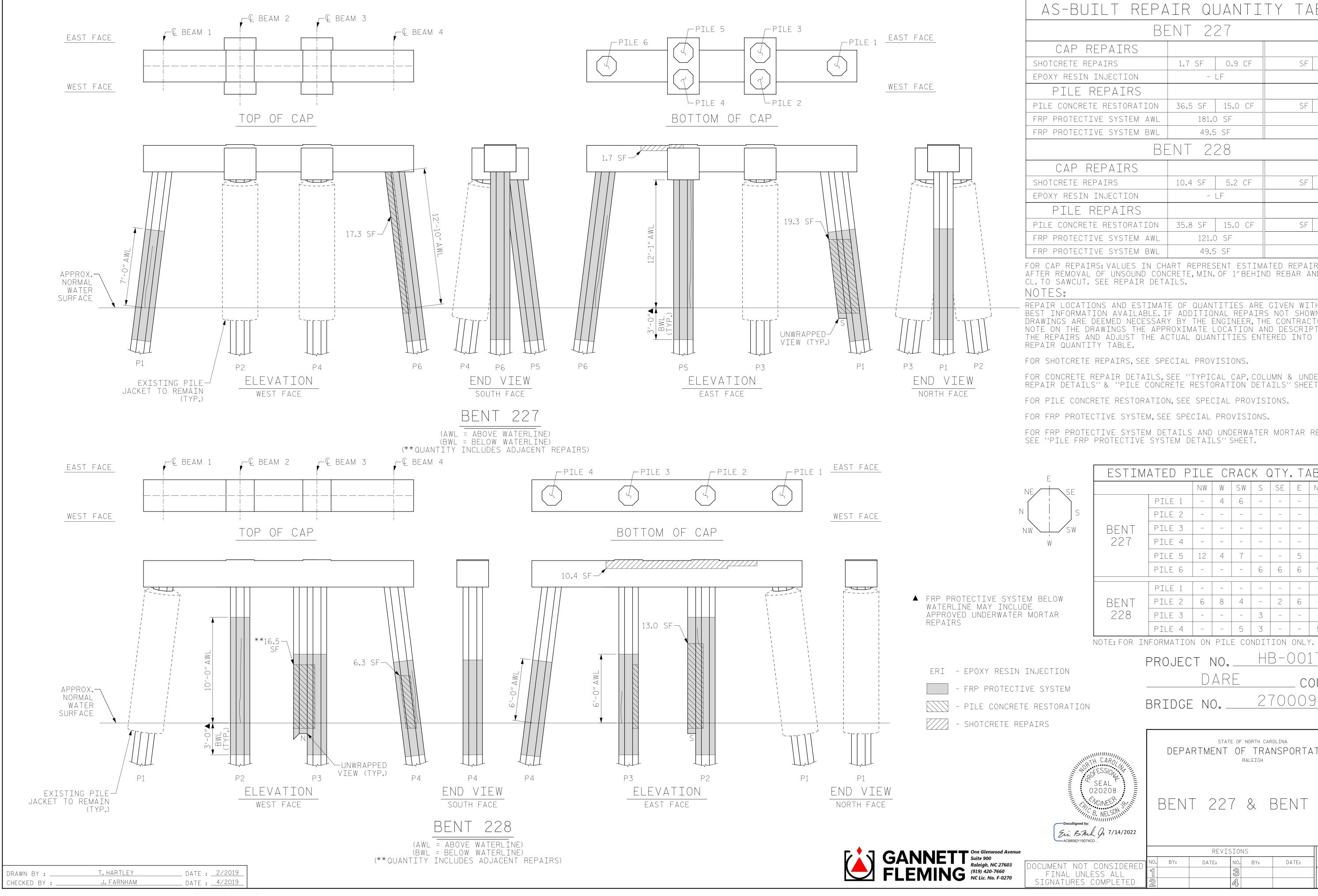
AS-BUILT REPAIR QUANTITY TABLE SF 1.7 SF | 0.9 CF PILE CONCRETE RESTORATION | 36.5 SF | 15.0 CF SF 181.0 SF 49.5 SF BENT 228 SF 10.4 SF | 5.2 CF
