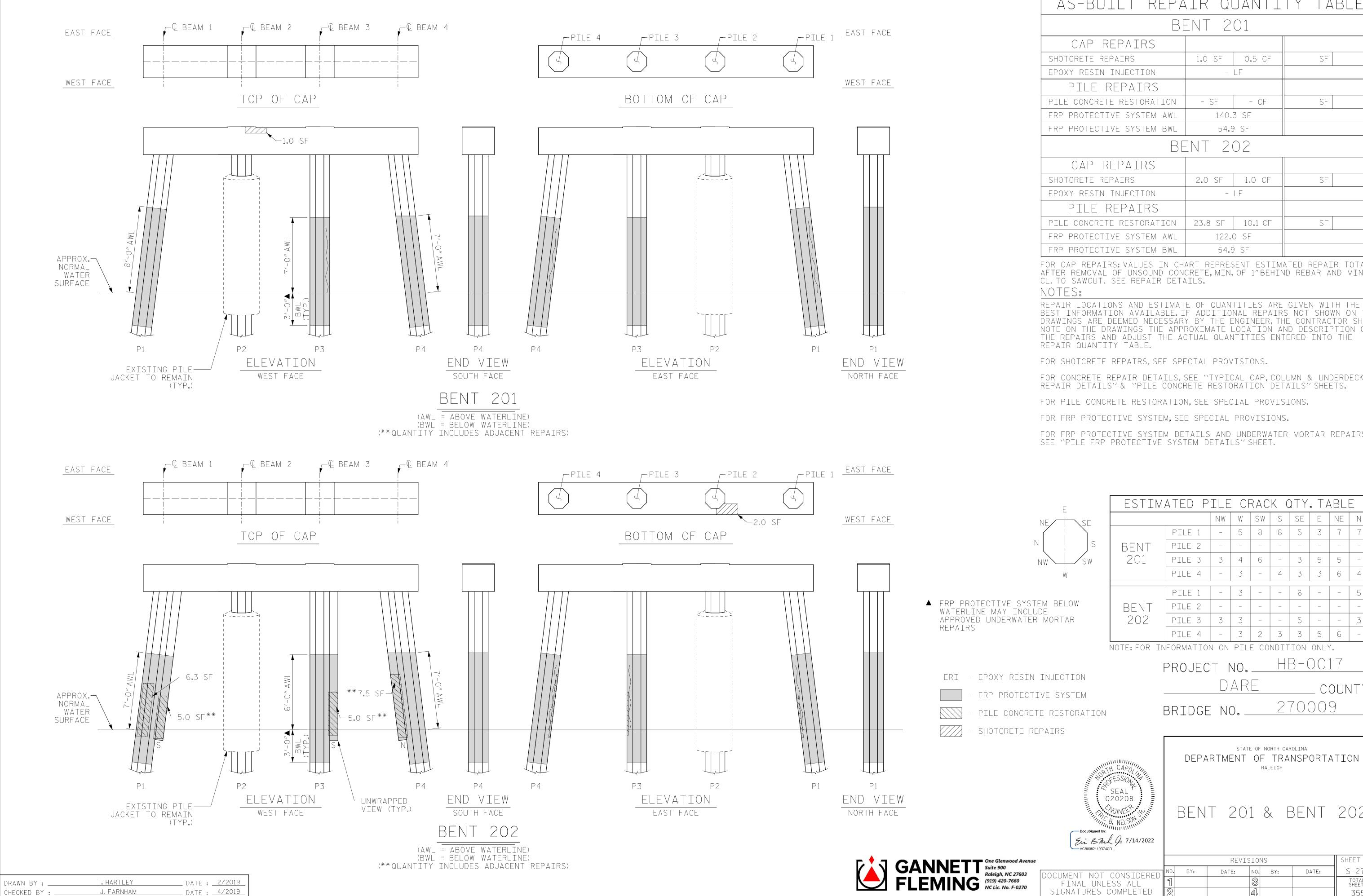
AS-BUILT REPAIR QUANTITY TABLE BENT 201 SF 1.0 SF | 0.5 CF - LF SF - SF 140.3 SF 54.9 SF BENT 202 SF 2.0 SF 1.0 CF - LF PILE CONCRETE RESTORATION 23.8 SF | 10.1 CF SF 122.0 SF
