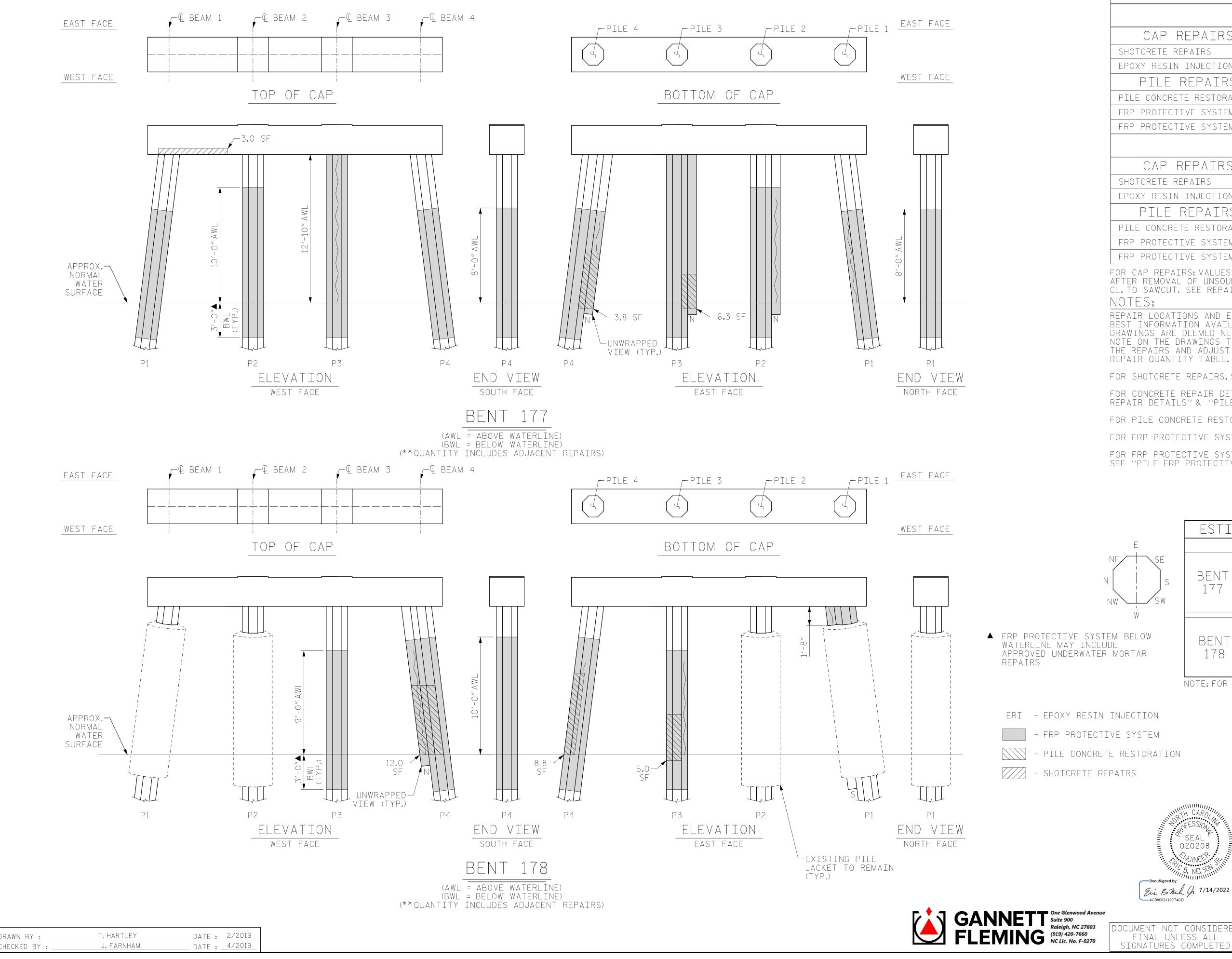
AS-BUILT REPAIR QUANTITY TABLE BENT 177 CAP REPAIRS SHOTCRETE REPAIRS 3.0 SF | 1.5 CF SF EPOXY RESIN INJECTION - LF PILE REPAIRS SF PILE CONCRETE RESTORATION 10.1 SF | 4.3 CF FRP PROTECTIVE SYSTEM AWL 236.9 SF FRP PROTECTIVE SYSTEM BWL 73.2 SF DENT 170
