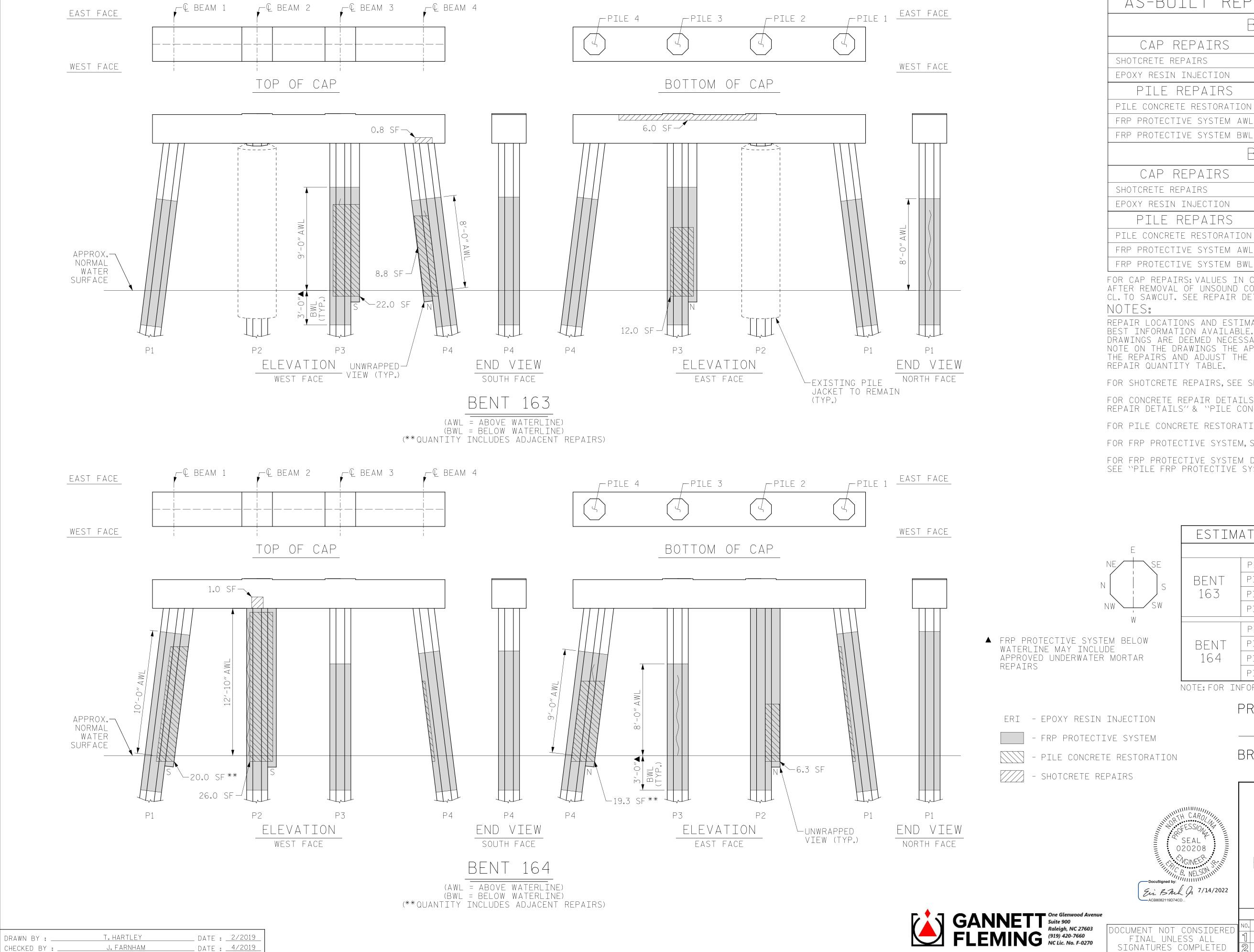
AS-BUILT REPAIR QUANTITY TABLE BENT 163 CAP REPAIRS SHOTCRETE REPAIRS SF 6.8 SF | 3.4 CF EPOXY RESIN INJECTION - LF PILE REPAIRS SF PILE CONCRETE RESTORATION 42.8 SF | 17.1 CF FRP PROTECTIVE SYSTEM AWL 152.5 SF FRP PROTECTIVE SYSTEM BWL 54.9 SF BENT 164 CAP REPAIRS 0.5 CF SF SHOTCRETE REPAIRS 1.0 SF EPOXY RESIN INJECTION - LF PILE REPAIRS SF PILE CONCRETE RESTORATION 71.6 SF | 30.0 CF
