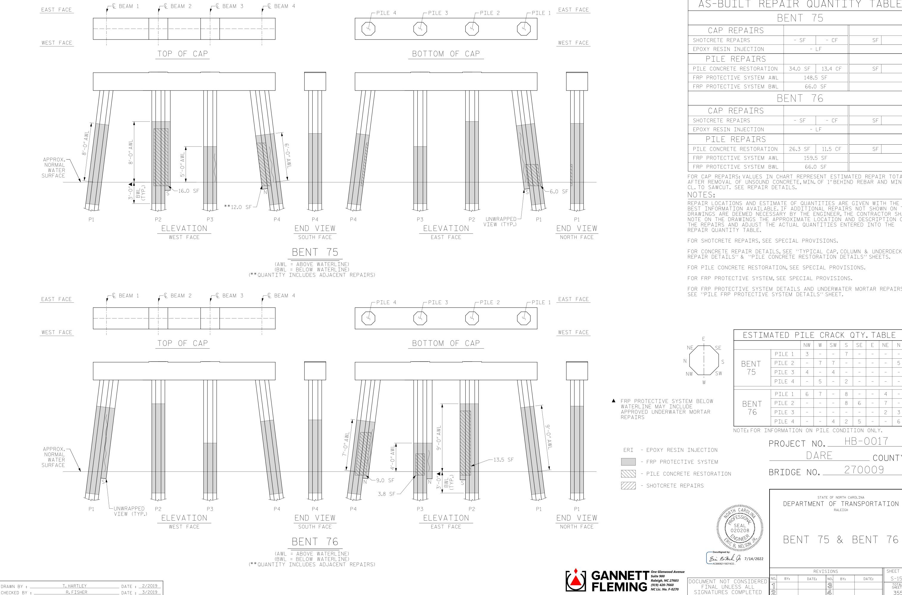
AS-BUILT REPAIR QUANTITY TABLE BENT 75 SF - SF - CF - LF PILE REPAIRS PILE CONCRETE RESTORATION | 34.0 SF | 13.4 CF SF FRP PROTECTIVE SYSTEM AWL 148.5 SF FRP PROTECTIVE SYSTEM BWL 66.0 SF BENT 76 SF - SF - CF - LF
