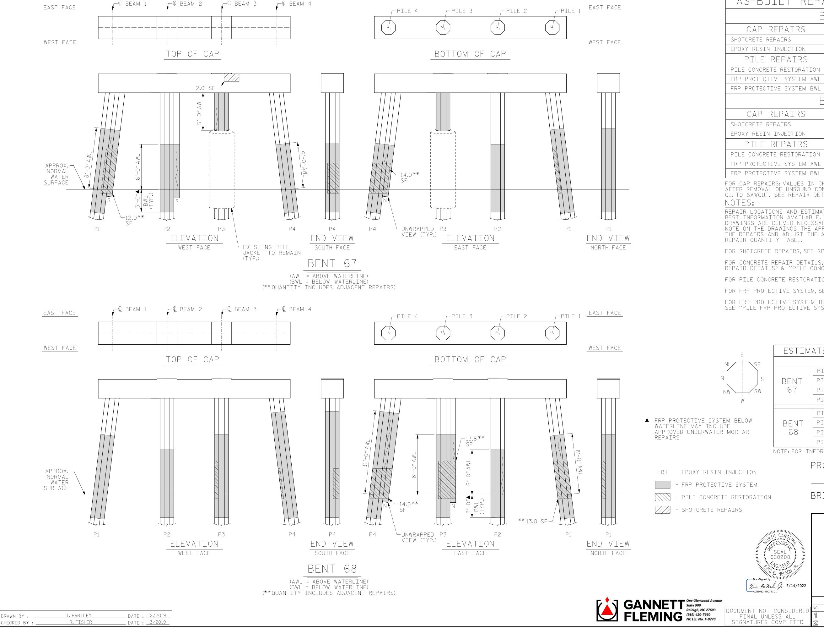
AS-BUILT REPAIR QUANTITY TABLE BENT 67 CAP REPAIRS SHOTCRETE REPAIRS SF 2.0 SF | 1.0 CF EPOXY RESIN INJECTION - LF PILE REPAIRS SF PILE CONCRETE RESTORATION | 26.0 SF | 9.9 CF FRP PROTECTIVE SYSTEM AWL 138.4 SF FRP PROTECTIVE SYSTEM BWL 49.5 SF BENT 68 CAP REPAIRS SF SHOTCRETE REPAIRS - SF - CF
