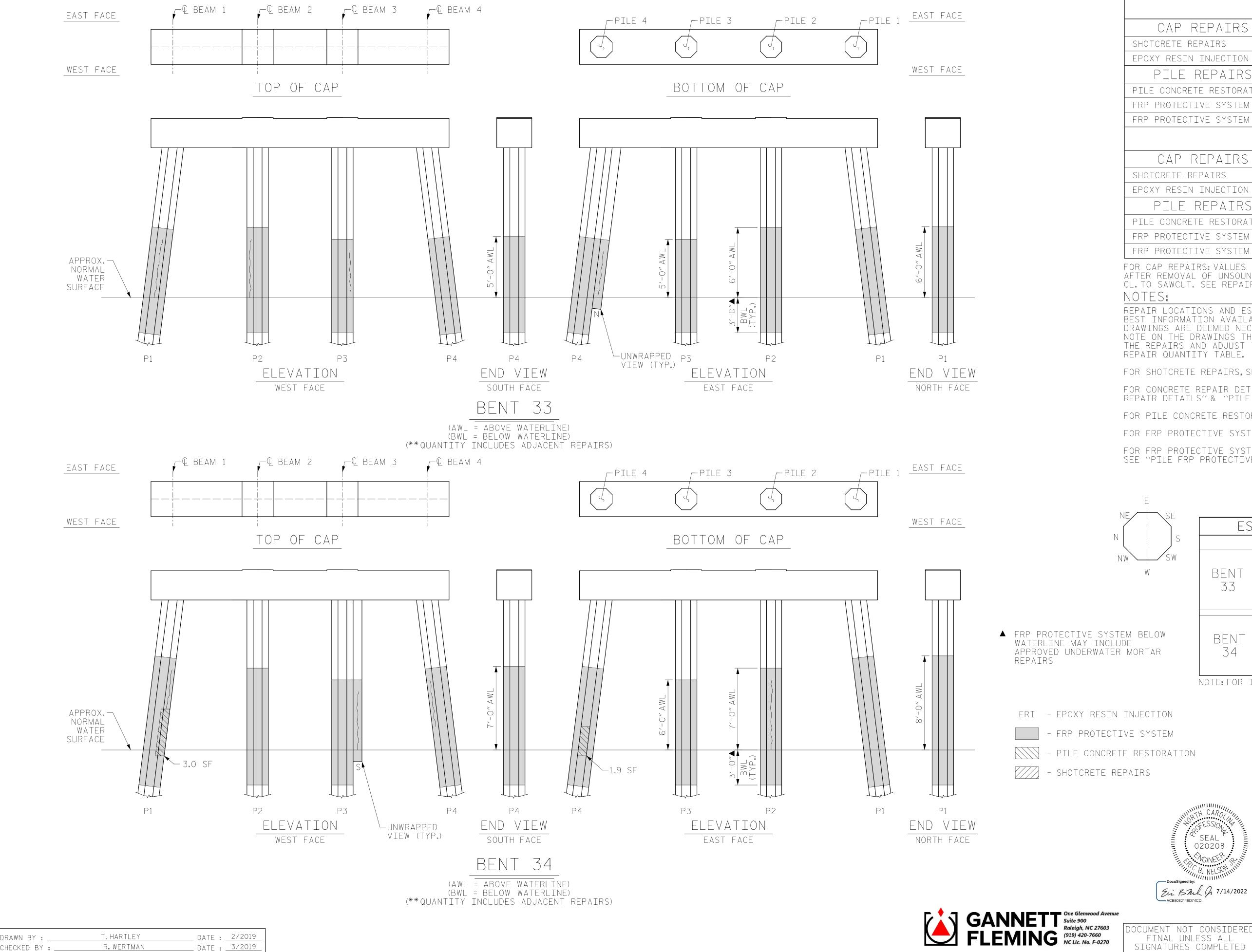
AS-BUILT REPAIR QUANTITY TABLE BENT 33 CAP REPAIRS ESTIMATE SHOTCRETE REPAIRS SF - SF - CF EPOXY RESIN INJECTION - LF PILE REPAIRS ESTIMATE SF PILE CONCRETE RESTORATION - SF | - CF FRP PROTECTIVE SYSTEM AWL 121.9 SF FRP PROTECTIVE SYSTEM BWL 66.0 SF RENT 3/
