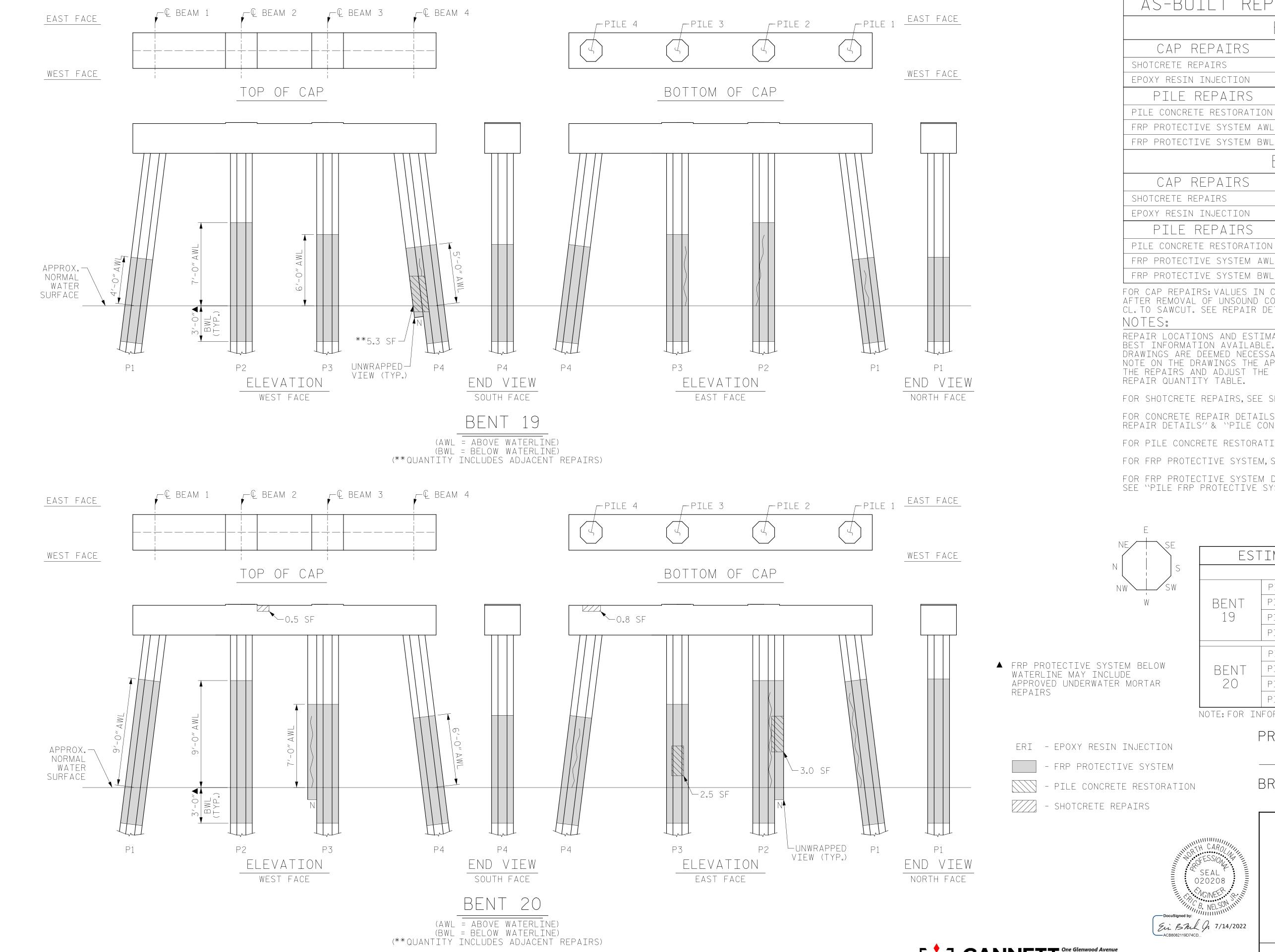
AS-BUILT REPAIR QUANTITY TABLE BENT 19 CAP REPAIRS ESTIMATE SF SHOTCRETE REPAIRS - SF - CF EPOXY RESIN INJECTION - LF PILE REPAIRS ESTIMATE SF PILE CONCRETE RESTORATION 5.3 SF | 2.2 CF FRP PROTECTIVE SYSTEM AWL 121.5 SF FRP PROTECTIVE SYSTEM BWL 66.0 SF BENT 20 CAP REPAIRS ESTIMATE SF SHOTCRETE REPAIRS 1.3 SF | 0.7 CF
