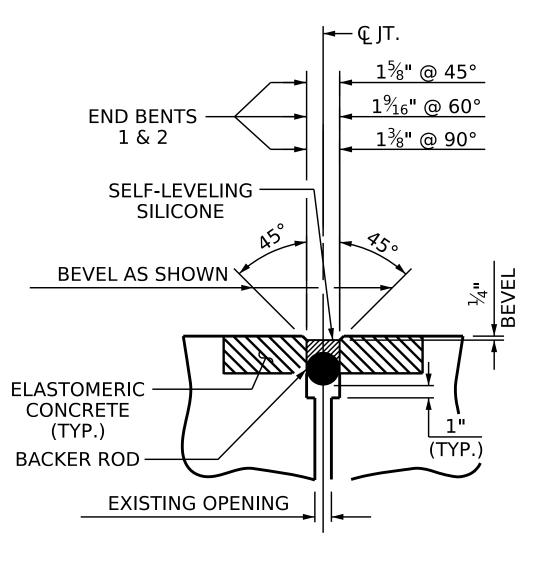
PROPOSED JOINT SEAL DETAIL
