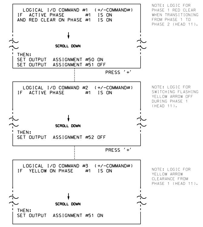
LOGIC I/O PROCESSOR PROGRAMMING COMPLETE
