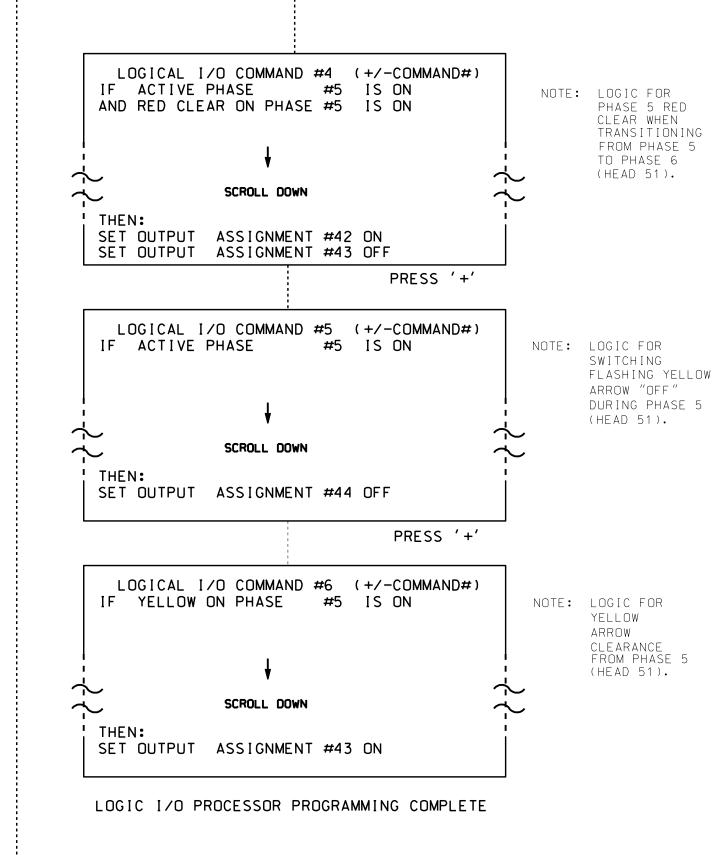
OUTPUT REFERENCE SCHEDULE OUTPUT 42 = Overlap C Red OUTPUT 43 = Overlap C Yellow OUTPUT 44 = Overlap C Green OUTPUT 50 = Overlap A Red OUTPUT 51 = Overlap A Yellow OUTPUT 52 = Overlap A Green
