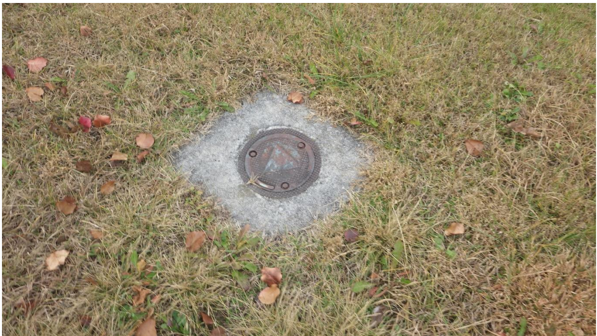
Older Monitoring well
